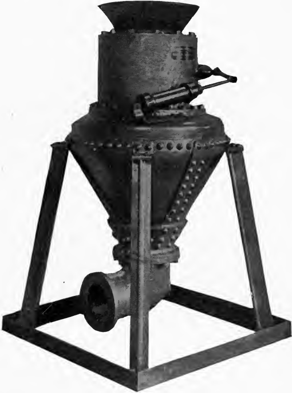
FIG. 103.—The Pneumatic Concrete Mixer. (Concrete Mixing & Placing Co.)
