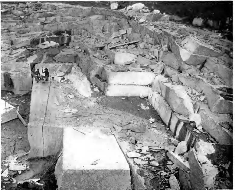
FIG. 13.—Spire of Granite Separated from Rock Mass on all Sides Except One End. Horizontal Joints of Rock Mass Are Clearly Shown.
