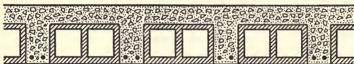
FIG. 42.—Hollow Block Fillers in Concrete Floors.
