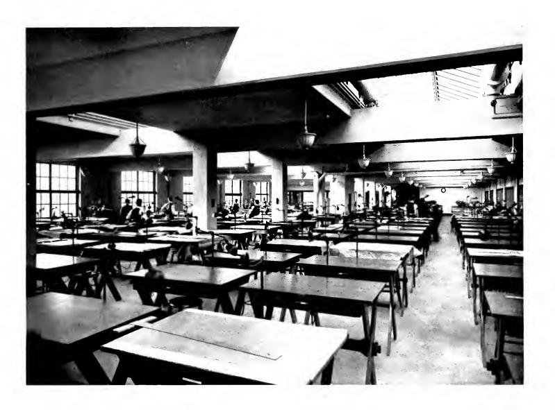
STUDENTS in the two Mechanical Engineering drafting rooms work under skylights in the roof, large windows also admitting a generous supply of daylight. The semi-indirect electric lighting system supplemented by desk lights permits work to continue during the evening when necessary.
