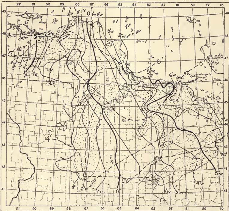
FIG 61 Lines of equal magnetic variation for 1905 giving the number of degrees that the compass points east and west of true north by the solid lines and the change in this variation per year by the dotted line, west variation increasing, east diminishing
