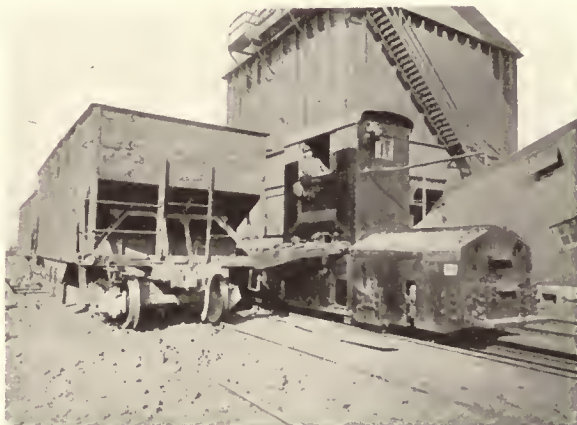
G-E Pusher Locomotive Designed for Spotting Cars Over Bins or Hoppers on Unloading Docks.
