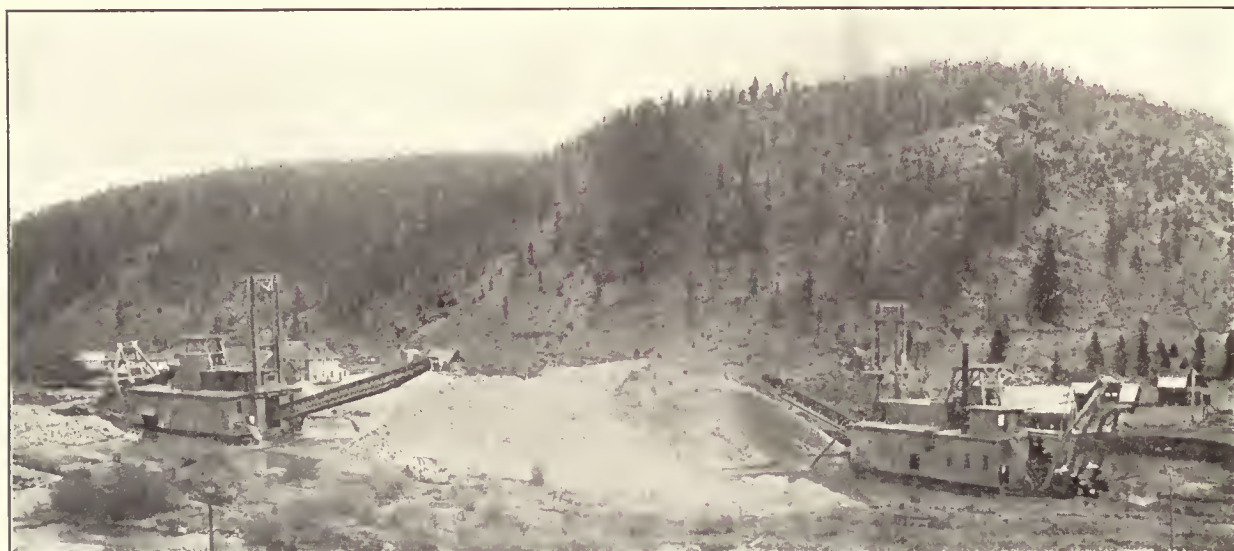
Two Placer Dredges at Work. Elevator or Dredging End Shown at Right, Disposal End at Left
