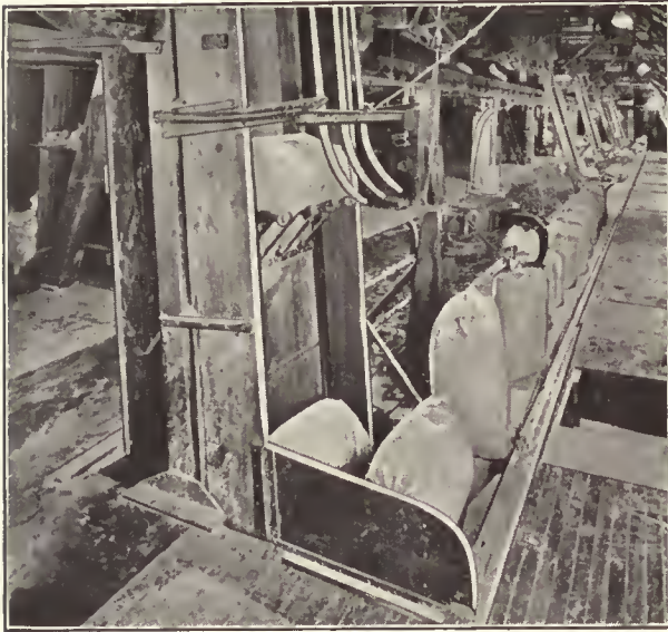
Belt Elevator with Automatic Feed
