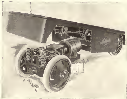
Complete Power Plant Being Installed in a High Load-Carrying Truck.
