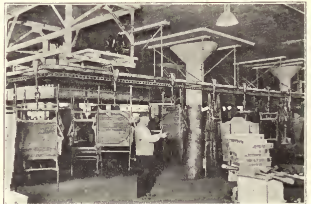
The Overhead Conveyor Saves Floor Space
