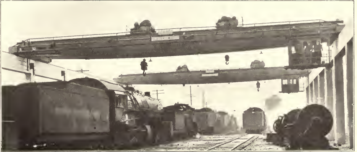
Two Chesapeake Electric Traveling Cranes Operating in a Railroad Yard.
