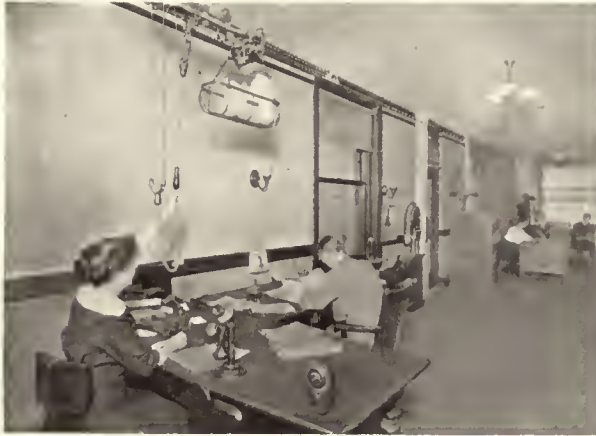
The Lamson wire line conveyor carries letters, folders, orders, requisitions, and all kinds of papers between desks, departments and offices.
