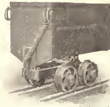
Fig. 403. Rotary Dump Car. Designed for mine work, in tunnels and other services where small over-all dimensions are an important feature.
