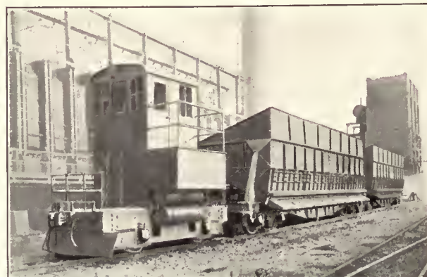
Electric Locomotive and Coke Cooling Cars
