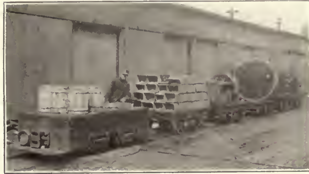
Storage Battery Platform Car
