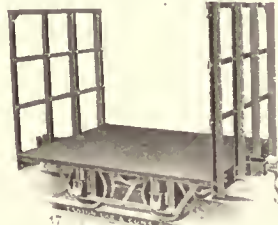
Fig. 147. Sugar Cane Car. All steel with end racks. We build a complete line of steel sugar cane cars to meet any requirement or specification.
