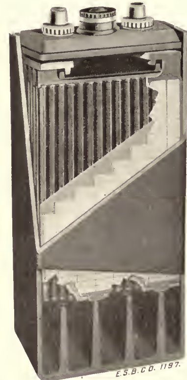
Cut-a-way Cell Showing New Construction — Positive Plates and Their Supporting Ribs; Negative Plates and Their Supporting Ribs; With Separators Extending Below All Plates.
