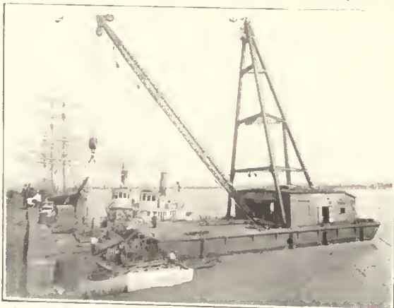
"A" Frame Barge Derricks, 5 to 150 Tons Capacity.
