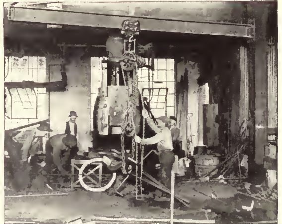
Cyclone Shock Absorber Hoist Suspended from Matchless Trolley Serving a Trip Hammer.
