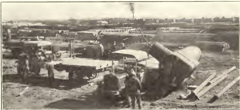
The White winch which may be had on 2, 3-3/4 or 5-ton models saves time and man-power in handling materials which have both bulk and weight. Above, an oil field boiler is being loaded upon a 5-Ton White with platform body.
