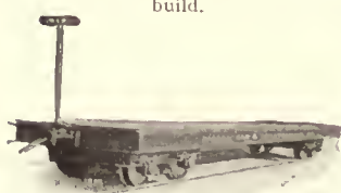
Fig. 1533. Special Double Truck Platform Car. Built to meet any specific requirements, in any desired size. Both with and without brakes.
