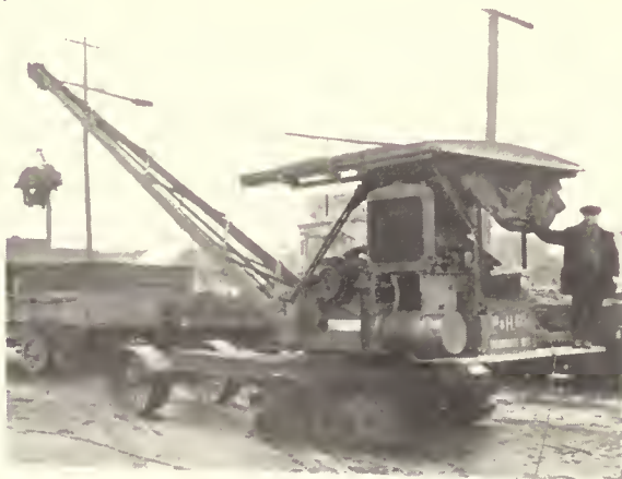
P & H Type 205 Crane with magnet unloading pig iron.
