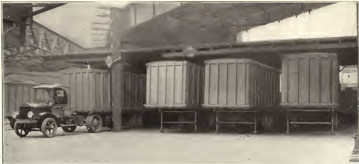
Semi-Trailers Eliminate Waiting Time of Truck-Tractors
