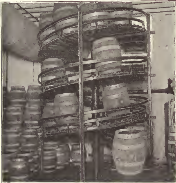
Spiral Provides Temporary Storage
