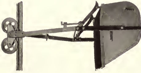
Self-Dumping and Self-Righting Bucket for Reversible Tramway
