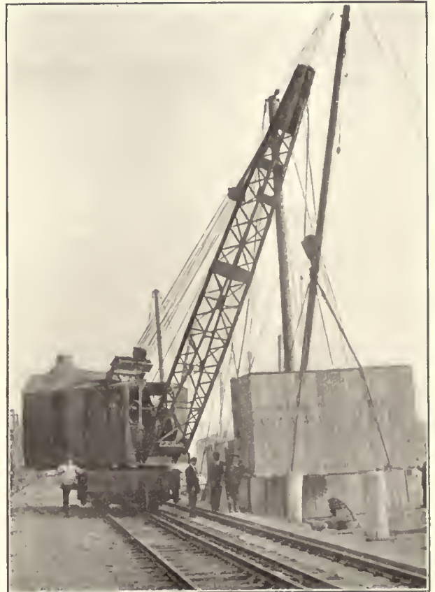
Steam Locomotive Crane Handling Heavy Freight from Car to Lighter for Export. Equipped with Shackle, Chains and Rope Slings
