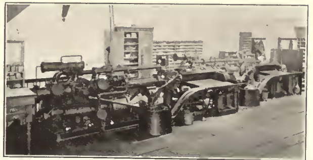
Pneumatic Package Conveyor
