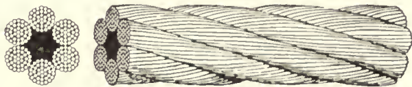
Special Flexible Hoisting Rope—One-Size Wire
