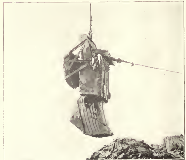
Hinged-Bail Back-Gate Drag-Line Bucket Dumping Soft Clay
