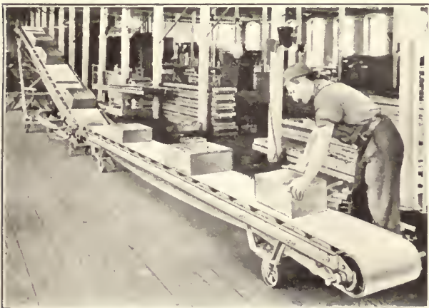
Automatic Transfer from Conveyor to Piler
