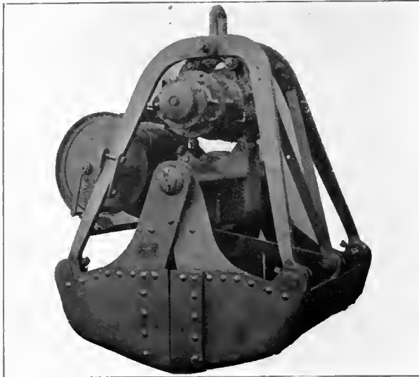
Electric Motor Clam-Shell Bucket with Electric Cable Take-Up Reel Attached. Single-Line Operation
