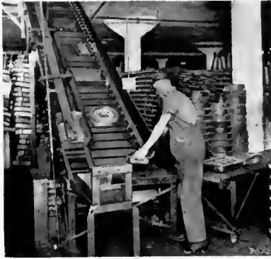
Inclined Apron Conveyor Delivering Automobile Parts from Basement Storage to First Floor Conveyor.
