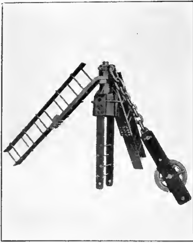
Cast Steel Stiff-Leg Derrick Mast Top with Wrought Iron Timber Straps and Chain Topping-Lift Connection
