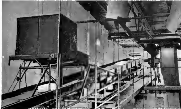
Merrick Conveyor Weightometer Weighing Material in Transit on a Belt Conveyor.
