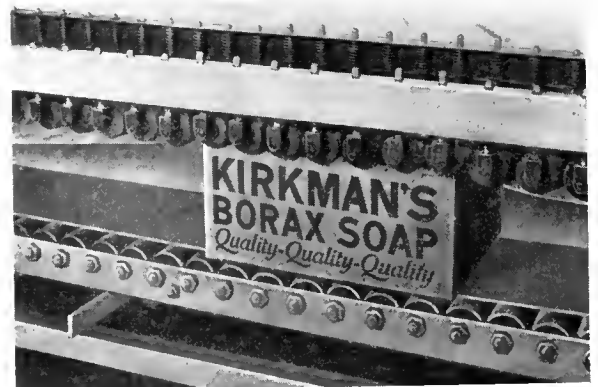
Showing the Flexible Pressure on the Top of the Case.
