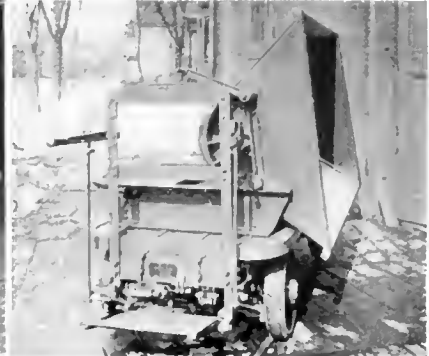
Crescent Dump Body Truck in Dumping Position.
