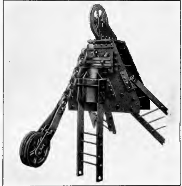
Structural Steel A-Frame Top with Single-Sheave Rooster and Chain Topping-Lift Connection
