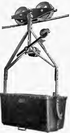
Bucket Carrier with Friction Grip
