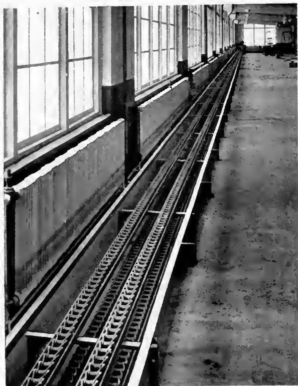
Lamson chain conveyor for carrying boxes of hobbins in textile mills. This type of conveyor is also used for carrying tote boxes, hampers, and other containers. National Spun Silk Co., New Bedford, Mass.
