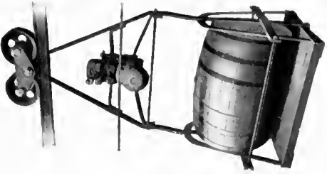
Platform Carrier for Barrels, Boxes, etc. Compression Grip
