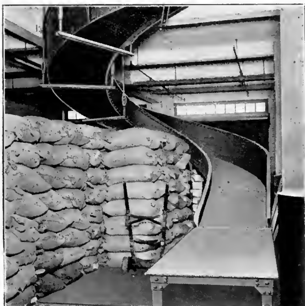
Saving Space Around Open-Center Spiral
