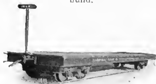
Fig. 1533. Special Double Truck Platform Car. Built to meet any specific requirements, in any desired size. Both with and without brakes.
