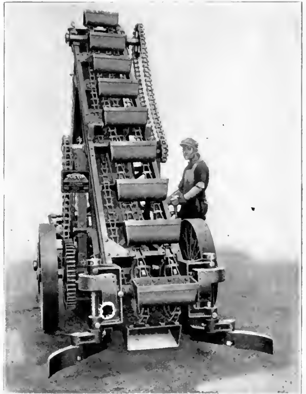
Austin Wagon Loader with Steel Feeding Arms Open
