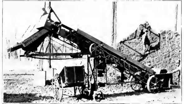
Portable Coke Loader.
