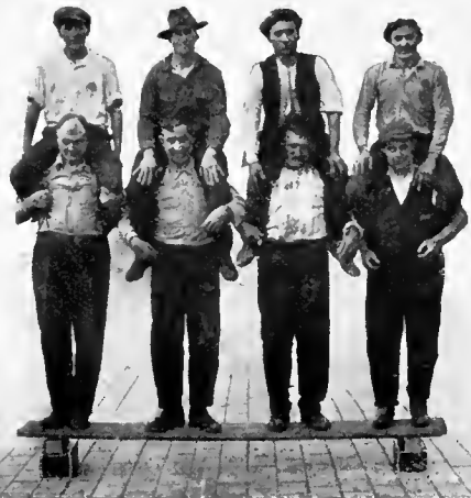
Two "Giant" Jars, in Which Exide-Ironclad Batteries Are Assembled, Supporting at Their Weakest Points, the Weight of 8 Men.
