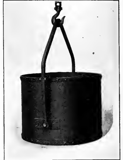
Self-Dumping Cylindrical Turnover Bucket with Rim Bail-Latch
