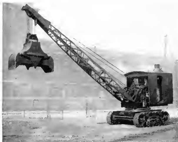
Brownhoist No. 2 Steam Locomotive Crane, Mounted on Brownhoist Creeper Trucks and Equipped with a Brownhoist 27 cu. ft. Grab Bucket for Handling Coal
