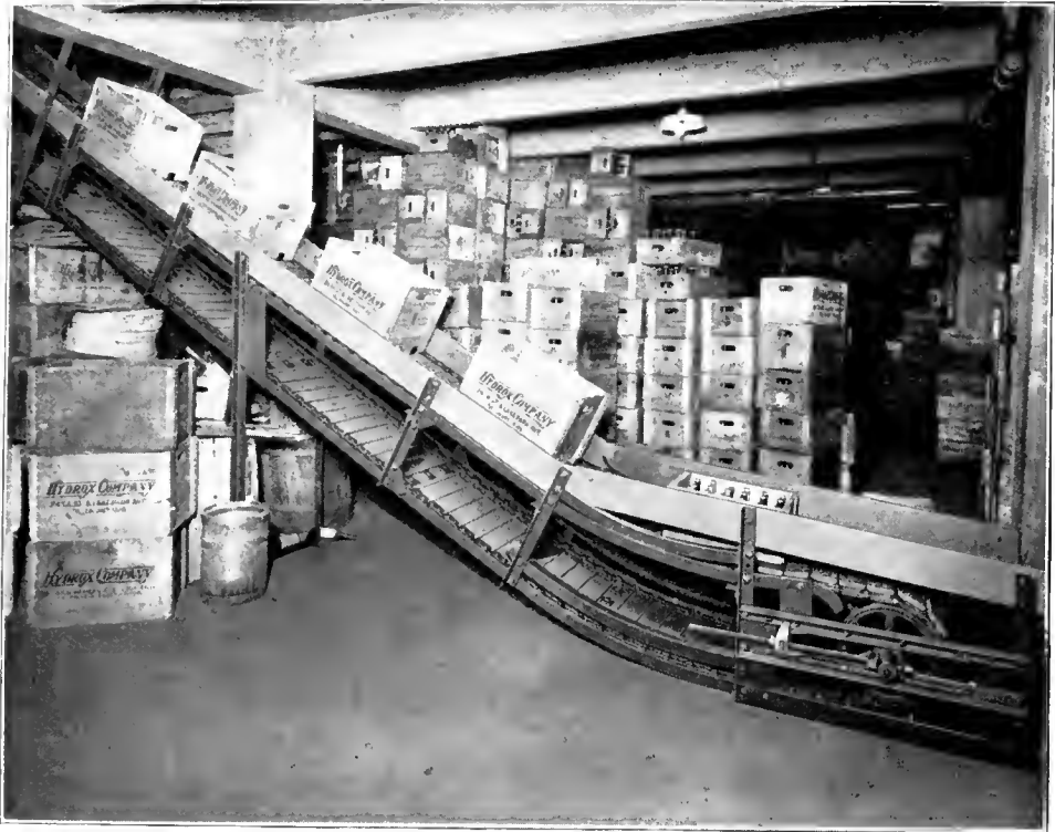
Inclined apron conveyor. One of many units in Hydrox Co.'s plant, Chicago, Ill.
