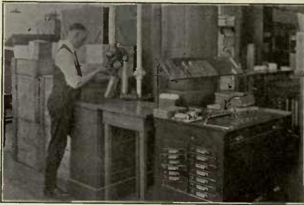
Shop Terminal of Pneumatic Conveyor
