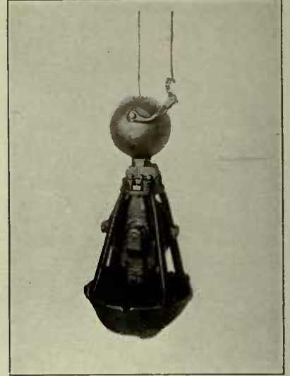
Dwarf Orange-Peel Bucket with Hammer Dropped and Bucket Closed
