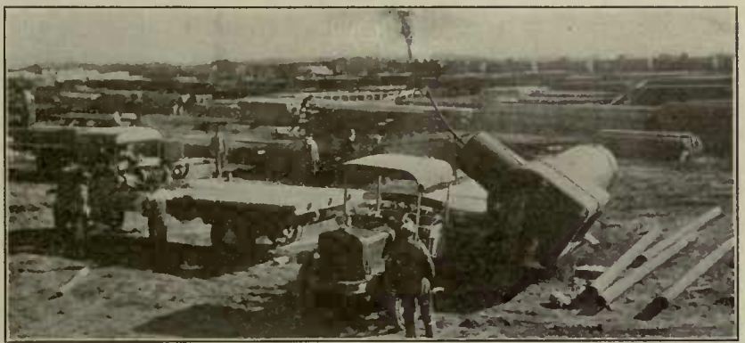
The White winch which may be had on 2, 3-3/4 or 5-ton models saves time and man-power in handling materials which have both bulk and weight. Above, an oil field boiler is being loaded upon a 5-Ton White with platform body.
