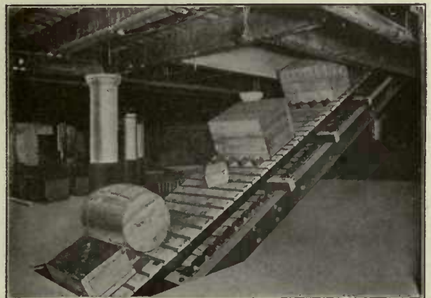
Direct Service Between Floors
