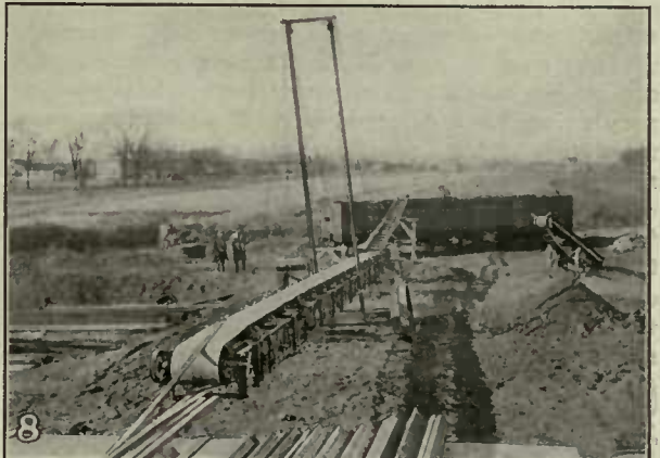
Applications of Portable Belt Conveyors: (1) Truck Loading; (2) Coal Storage; (3) Industrial Car Loading; (4) Gravel Pit; (5) Retail Coal Yard; (6) A Unit in a Conveyor Line; (7) Car Unloading; (8) Handling Lumber
