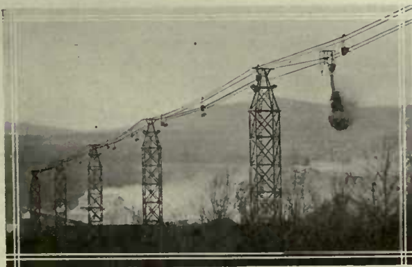
Leschen Automatic Tramway disposing of waste at an asbestos mine in Canada.
