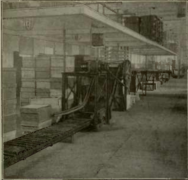
Extending Scope of Gravity Conveyor
