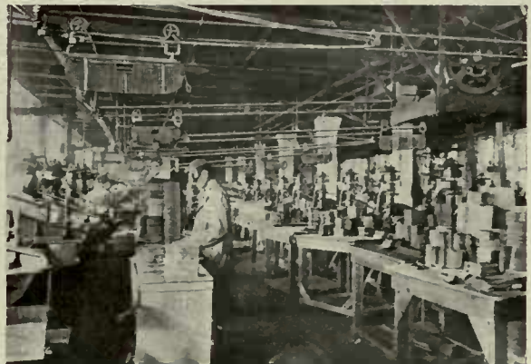
Lamson wire line conveyors in shoe factory carrying dies from die room to operators. They also carry tools, job tickets, time tickets, small parts, laboratory samples, etc. Weinbrenner Co., Milwaukee, Wis.
