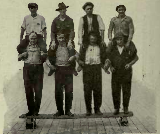
Two "Giant" Jars, in Which Exide-Ironclad Batteries Are Assembled, Supporting at Their Weakest Points, the Weight of 8 Men.
