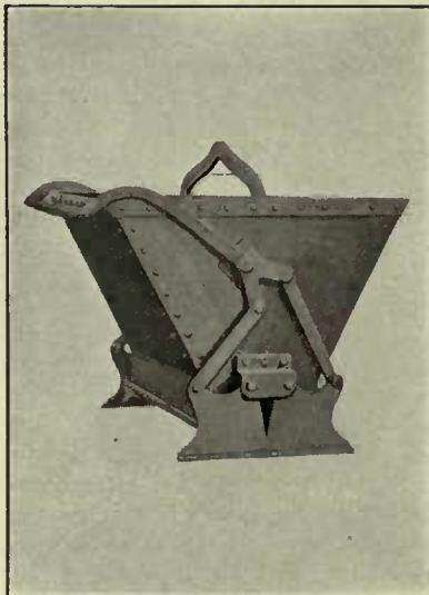
Controllable-Discharge Center-Hinged Bottom-Dump Bucket. Bell-crank Crossbar-Lever Operation
