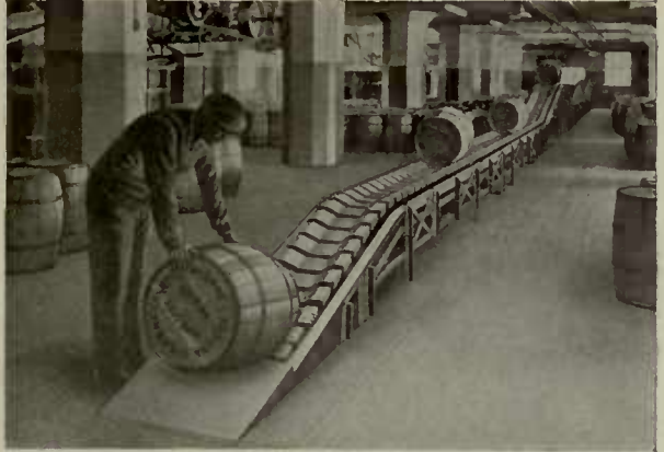
Lamson heavy duty slat conveyors are built in different types to carry barrels, cases, castings, hales, and other heavy loads. Revere Sugar Refinery, Charlestown, Mass.
