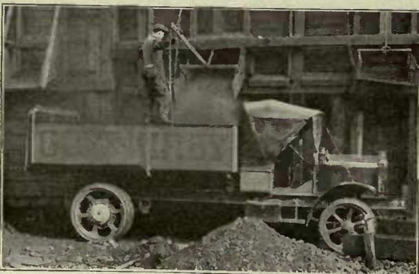
Coal, ashes or other bulk materials are quickly and easily loaded and unloaded when White Trucks with power dumping bodies are used.
