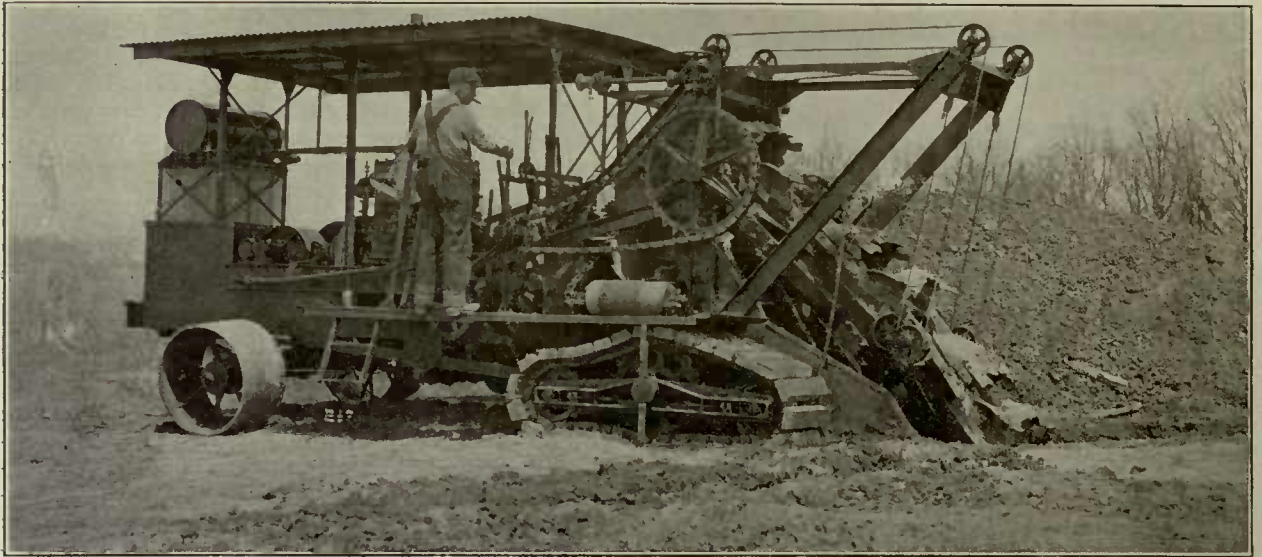
Endless-Chain Bucket Type Trenching Machine with Topping-Lift. Bucket Equipped with Side Cutters
