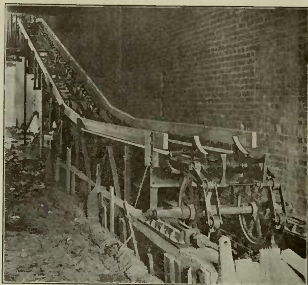
Barrel and Sack Elevator-Conveyor
