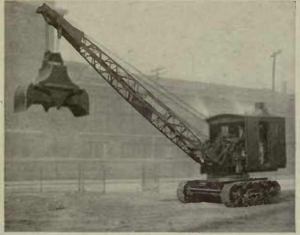
Brownhoist No. 2 Steam Locomotive Crane, Mounted on Brownhoist Creeper Trucks and Equipped with a Brownhoist 27 cu. ft. Grab Bucket for Handling Coal
