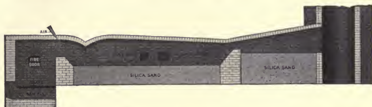
FIG. 85.—Longitudinal section of an air furnace.
