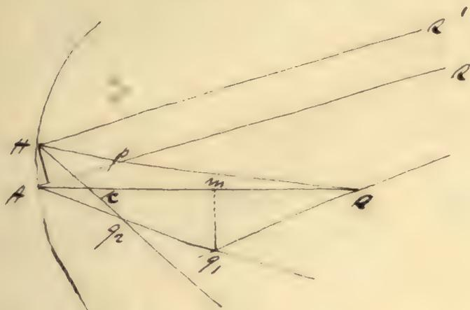
Let the axis of the incident pencil.  $Aq_1$  the axis of the reflected pencil - since the pencil consists of rays, the line thro' O. from the origin may be considered  $\perp$  to  $Aq_1$ .
