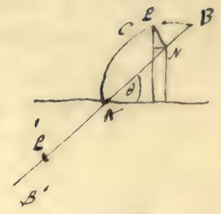
$B'B'$  is movable about  $A$  in a vertical plane, which also coincides with the plane of the  $\theta$ . Two particles  $a, b$  are placed one at  $B$  capable of moving along  $BCA$ . the other at  $B'$  capable of moving along  $AB'$ . determine the motion of each particle.
