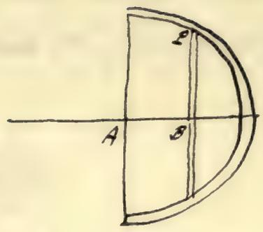
The moment of inertia of the annulus contained between planes  $\perp$  to the axis at a distance  $x$  and  $x + dx$  from A will be.
