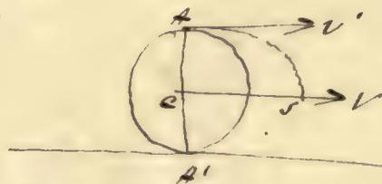
At  $A$  a molecule on the surface of the wheel would be at rest, at  $A$  its velocity would be in direct:  $A v'$  // to the horizontal plane, and  $= 2v$ .
