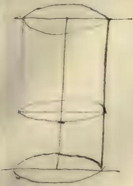
Let  $x =$  depth of the base of the cylinder below the surface of the fluid at a time  $t$ .
