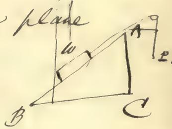
To find the pressure on the fulcrum of a lever kept at rest by any two pressures.
