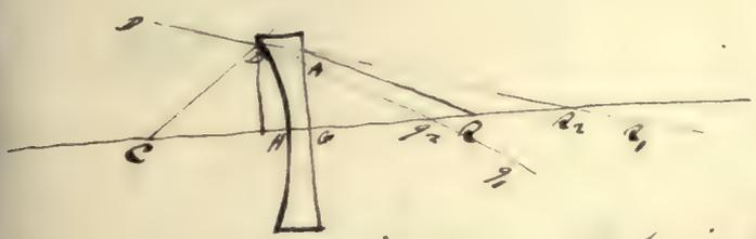
the origin of the pencil.  $g_2$  is the position after refraction at the first surf.  $g_1$  is the position after refraction at the second surf.
