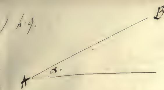
Let  $\alpha$  = inclination of the plane to the horizon. take BA for the axis of  $x$ .
