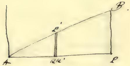
Then the mass of the thin circular sect. generated by the revolut. of  $PAA'$  about the axis of  $x$  ( $AA = x$   $AA' = x + dx = \rho dx \cdot \pi y^2$ )
