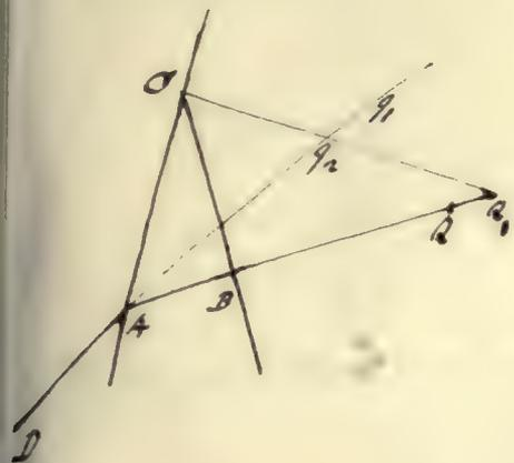
ABAD is the course of the axis of a pencil which is incident directly at B on the first surface of a prism. find its primary and secondary foci after refraction.
