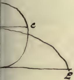
$AB$  the vertical side of a vessel filled with fluid.  $D$  an orifice.  $DE$  the course of the issuing stream.  $BCA$  a semicircle.
