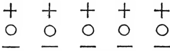
A DIAGRAM OF FIELDS OF FORCE AND NEUTRAL ZONE IN A BEAM
