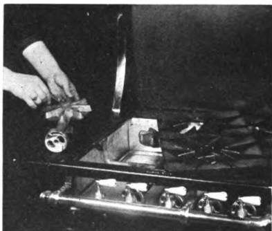
FIG. 6. Cleaning burner of gas stove.
