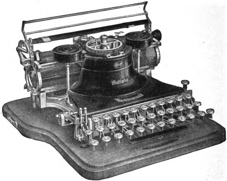
FIG. 146. Hammond interchangeable typewriter.
