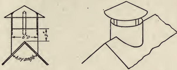
FIG. 242. ROOF CAP AND VENTILATOR
