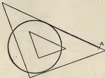
FIG. 372. TO CONSTRUCT A TANGENT TO A CIRCLE THROUGH A POINT WITH THE TRIANGLE
