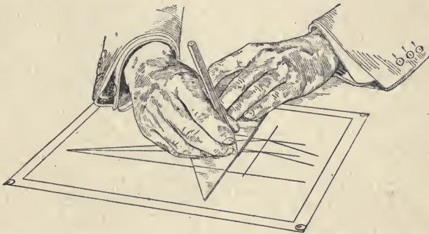
FIG. 13. DETERMINING THE WIDTH OF THE FACE OF THE CUBE
