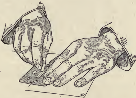
FIG. 139. USING THE ERASER AND SHIELD
