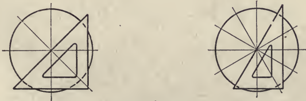
FIG. 210. DIVIDING A CIRCLE INTO 8 OR 12 PARTS WITH TRIANGLES
