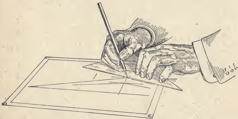
FIG. 12. SKETCHING THE ANGLES OF INCLINATION
