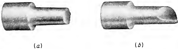
Fig. 10-5. Typical torsion failures. (a) Shear (ductile) failure; (b) tensile (brittle) failure.
