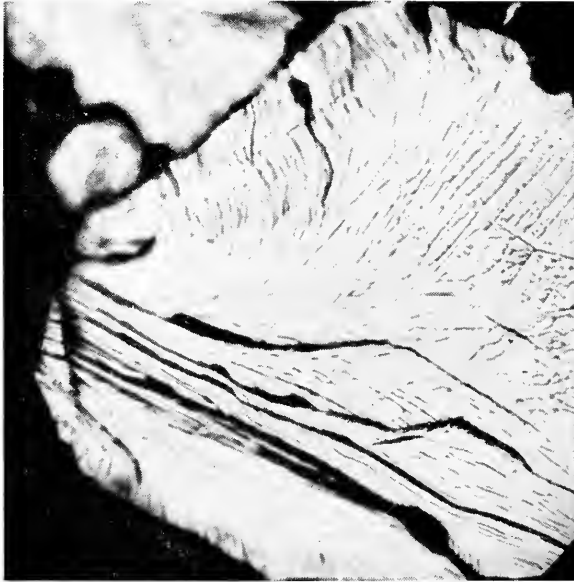
Fig. 7-6. Cleavage steps and river pattern on a cleavage surface.
