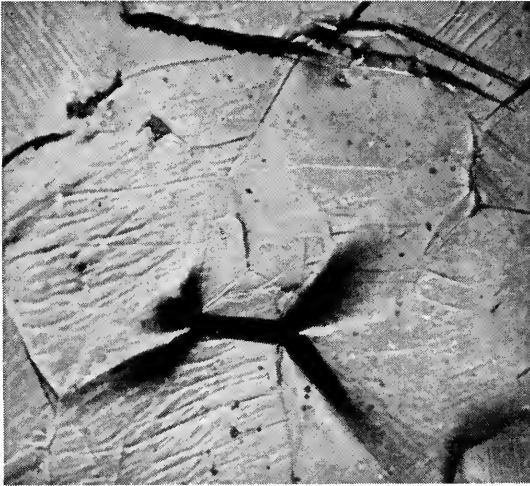
Fig. 7-4. Microcracks produced in iron by tensile deformation at -140^{\circ}\text{C} . 250 \times . (Courtesy G. T. Hahn.)
