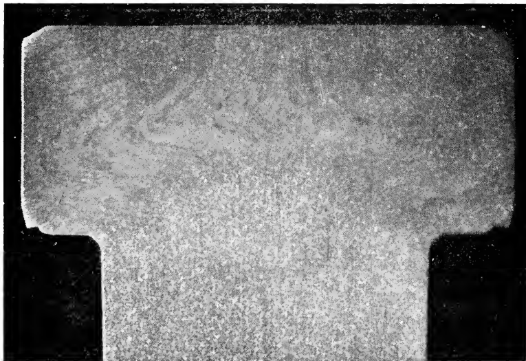
Fig. 17-3. Fiber structure in wrought product revealed by macroetching. 5 \times .
