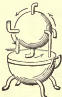
219. ORIGINAL FORM of the Æolipile or Hero's Steam Engine, 130 B.C. A reaction power, suitable for operation by the use of any gaseous or fluid pressure. The original type of several modern motors.
