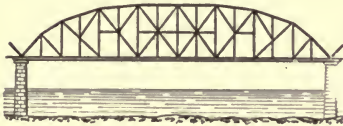
1491. ARCHED DECK TRUSS BRIDGE.—The arch takes the pressure and gives tension to the chord. Struts and tie rods give stability to the structure.
