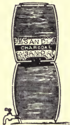
581. DOMESTIC FILTER.—Use two stone pots or jars, the bottom one being a water jar with side hole; if no faucet can be used, the top jar can be removed to enable the water to be dipped out. The top jar must have a hole drilled or broken in the bottom, and a small flower-pot saucer inverted over the hole. Then fill in a layer of sharp, clean sand, rather coarse.
