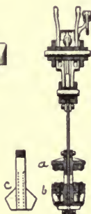
1599. CABLE GRIP FOR STREET RAILWAYS.— a , b , grip jaws and blocks; c , pull-up to throw the cable out of the jaws; d , d , frame plates; e , grip plate connected to b , and operated by the bell crank levers g , g ; f , f , pull-up attached to frame and disengaging pieces c , c .
