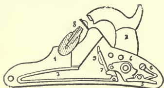
1638. GUN LOCK.—1, lock plate; 2, hammer; 3, mainspring; 4, tumbler; 5, sear or trigger lever; 6, sear spring.
