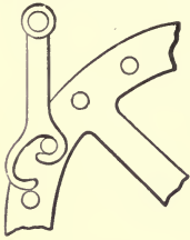
1056. INTERMITTENT MOVEMENT of a pin-wheel by the vibration of a hooked arm.
