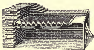
207. SHAKING AND TIPPING FURNACE GRATE.—The front and back sections can be shaken separately by the double connections and levers.
