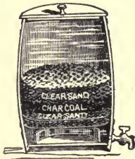
580. DOMESTIC FILTER.—To make a filter with a wine barrel, procure a piece of fine brass wire cloth of a size sufficient to make a partition across the barrel. Support this wire cloth with a coarser wire cloth under it and also a light frame of oak, to keep the wire cloth from sagging. Fill in upon the wire cloth about three inches in depth of clear, sharp sand, then two inches of charcoal
