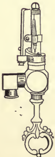
737. ELECTRIC GAS LIGHTER.—Turning on the gas brings the electrodes in contact, and breaks the contact, which produces a spark by closing and opening the battery circuit.
