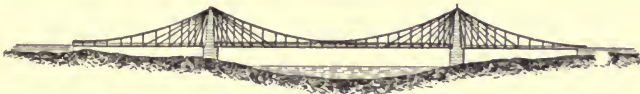
1508. SUSPENSION BRIDGE.—The Cincinnati bridge, "Roebling" system. Ten hundred and fifty-seven feet between piers.
