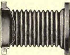
415. CORRUGATED EXPANSION COUPLING, "Wainwright's" model. A hard brass tube, corrugated, gives the tube a longitudinal elasticity to take up the expansion of steam pipes.
