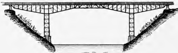
1505. CANTILEVER BRIDGE.—The ends, being anchored, balance all other parts on the piers. This cut shows the principle of Cantilever construction.
