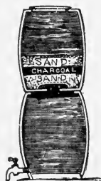
581. DOMESTIC FILTER.—Use two stone pots or jars, the bottom one being a water jar with side hole; if no faucet can be used, the top jar can be removed to enable the water to be dipped out. The top jar must have a hole drilled or broken in the bottom, and a small flower-pot saucer inverted over the hole. Then fill in a layer of sharp, clean sand, rather coarse.
