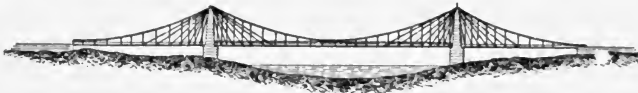
1508. SUSPENSION BRIDGE.—The Cincinnati bridge, "Roebling" system. Ten hundred and fifty-seven feet between piers.
