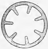
202. "SERVES" BOILER TUBE.—The projecting ribs enlarge the area of the fire surface of the tube.
