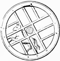
1534. HORSE-POWER MACHINE.—An endless chain and rollers, with a slatted platform, roll over a sprocket-wheel driving shaft. The walking platform is elevated to an angle of about 15^{\circ} .
