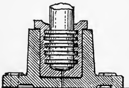
1282. COLLAR BEARING AND STEP for a vertical shaft. The thrust sleeve of bronze is split and should have a key to prevent rotation.
