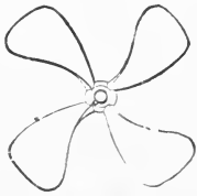
822. OUTWARD THRUST PROPELLER WHEEL.—The blades pitch forward to throw the water outward as well as backward, to increase the thrust or power of the wheel.
