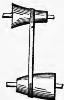
90. CURVED CONE PULLEYS, for variably in- creasing or decreasing speed by traversing the belt.
