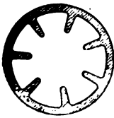
202. "SERVES" BOILER TUBE.—The projecting ribs enlarge the area of the fire surface of the tube.
