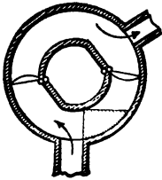
543. One of the early forms of Rotary Pumps. Only suitable for free flow to the pump. Will not lift. Obsolete.
