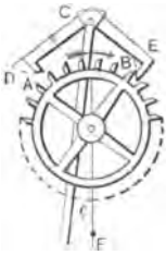
1171. DEAD-BEAT CLOCK ESCAPEMENT.—The face of teeth is slightly pitched forward. The stop-faces of the pallets A, B are concentric with the axis, which gives the dead-beat stop.
