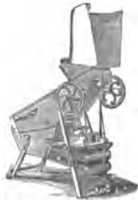
1245. GOLD SEPARATOR; dry process. A bellows furnishes an air blast, which separates the fine sand and dust from the gold on the riffle screen and blows the dust away.
