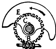
920. RELEASE CAM.—Uniform motion is communicated to the gear wheel, B, fixed on its shaft with a pin at C. The cam is loose on the shaft, with a stop section to meet the pin at C. The lever d has a spring and a roller on the cam. The lever d is raised by the motion of the cam until its straight face reaches the roller, when the lever falls suddenly, throwing the cam forward.
