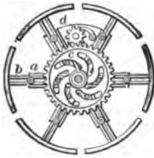
934. EXPANDING PULLEY.—The sectional rim pieces with their arms have a radial sliding joint on the hub arms, and are moved out or in by pins projecting into the spiral slots on the central spur-gear wheel. The movement of the wheel c , by turning the ratchet pinion d , moves all the sections of the pulley equally.
