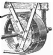
1325. BELT HOLDER, "Wellington" model. Does away with a loose pulley. The belt is guided on to a set of rollers in a fixed frame at the side of the driving pulley. Saves time and avoids danger in putting on belts.
