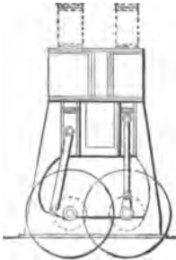
233. COMPOUND ENGINES for twin screws. There may be one or two pair of compound cylinders. The dotted lines represent cylinders of the tandem model.
