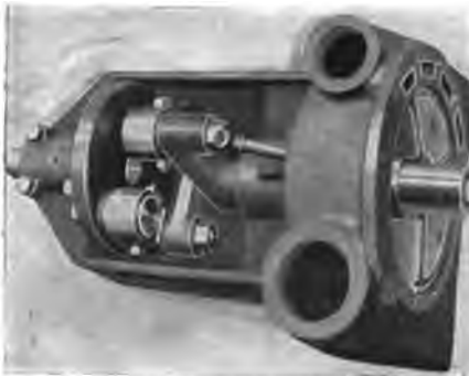
357. Shows the crank end of the vibrating shafts with the link connections. The steam port is in the cylinder head, which is the steam chest. During one-half of a fly-wheel revolution one of the sectors makes a large angular movement, while the other makes a relatively small angular movement, and during the second
