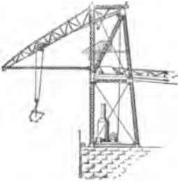
1213. ELEVATOR TOWER with inclined boom. The bucket is lifted to the trolley by the double tackle, drawn up the incline, and the load dumped automatically into a car.
