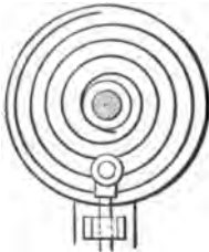
1081. SPIRAL-GROOVED FACE PLATE, for feed motion. Obsolete; but useful for irregular motion, in which the spiral grooves may be wavy or zigzag.
