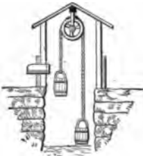
524. WELL PULLEY AND BUCKETS.—Buckets are balanced empty.
