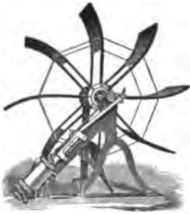
1208. STEAM-DRIVEN VENTILATING FAN.—Type of those used in the coal-mining districts. The fan wheel may be encased in an iron or wooden shell.
