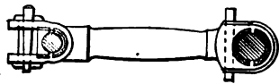
463. LINK OR CONNECTING ROD, with adjustable brasses. Keys inside and outside of pins.
