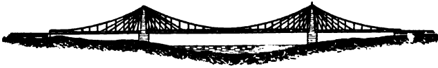
1508. SUSPENSION BRIDGE.—The Cincinnati bridge, "Roebing" system. Ten hundred and fifty-seven feet between piers.
