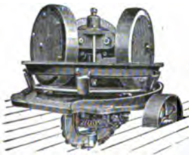
1240. PULVERIZING BALL AND PAN MILL.—The pan is continually tilted by being swung around the vertical centre, rolling the ball down the slope side of the pan.
