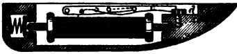
1573. SEWING-MACHINE SHUTTLE.—The thread is rove in the holes in the tension spring, which is made adjustable by the notch cam d .
