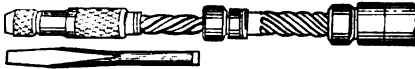
1392. DOUBLE-ACTING SCREWDRIVER.—The inside spindle has a left-hand screw, the outside hollow spindle a right-hand screw; and both with nuts that can lock either spindle by screwing to the thread on the
