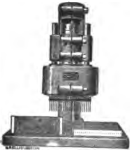
1359. MULTIPLE DRILLING MACHINE, for close drilling or perforating plates. Drills are operated close together by converging spindles.
