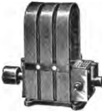
731. SPARKING DYNAMO, or generator for a marine gasoline engine. Permanent horseshoe magnets, with an armature revolved by a belt from the fly-wheel of the engine. With a true rim on the fly-wheel, the pulley of the generator may be covered with leather or rubber and pressed lightly against the rim of the fly-wheel.
