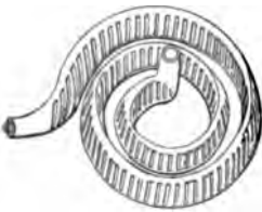
201. "SERPOLLET'S" STEAM GENERATOR, showing the corrugated flattened tube coiled into a volute. The width of the internal space is less than one-eighth of an inch.
