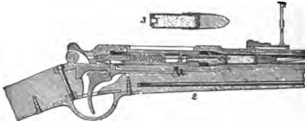
1642. CHASSEPOT GUN.—A needle gun. The cartridge is inserted by hand; the plunger runs forward and is locked by turning into a notch. Centre fire.
