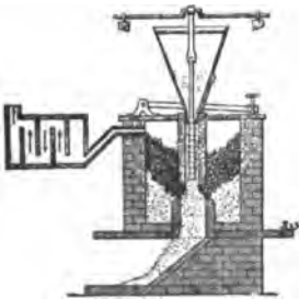
750. ELECTRIC FURNACE, "Cowles" hopper model. The upper electrode is a vertical carbon tube fixed to the hopper. The lower electrode is a larger carbon tube fixed to the furnace floor. The tubes are banked with carbon and lime. The charge is fed down from the hopper by a barbed rod, reciprocated by a crank. The gases generated are drawn off through a condenser.
