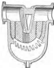
405. STEAM SEPARATOR, in line for horizontal pipes. The corrugated surface catches the water of condensation, which falls through the grating to the recess below. "Austin" model.
