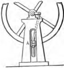
290. PARALLEL MOTION by guide bars in the frame of a vertical engine, with connecting piston rod and crank. Cross-head sliding in a slot in the frame. Old.
