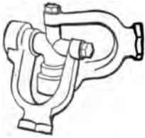
1384. FLEXIBLE UNIVERSAL STEAM JOINT.—“Hampson” model. The steam flows through the thick arms of the Y's, which have ground joints.
