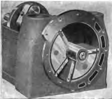
356. VIBRATING PISTON ENGINE, "Parson's" model. Two sector pistons vibrating in a cylinder. One sector is fast on a central solid shaft, the other is fast on a concentric hollow shaft. At the other end of each shaft is a crank and link connection to a wrist pin at opposite positions on a
