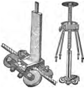
1597. CABLE RAILWAY GRIP.—Friction sheaves are drawn tightly on the cable by a vertical bar in the frame plate. Friction is increased by further tightening the grip wheel.
