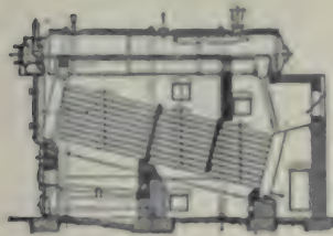
184. "BABCOCK & WILCOX" WATER TUBE BOILER.—Inclined straight tubes expanded in vertical steel headers, connected to a steam drum above. Partitions re-pass the flame through the tube spaces.
