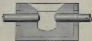
747. OPEN TOP ELECTRIC FURNACE.—A cavity in a box of refractory material with holes on each side through which the insulated carbon electrodes are inserted.
