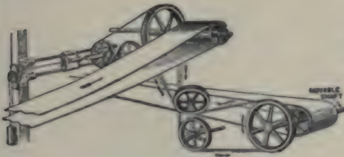
63. ROPE TRANSMISSION to a movable shaft at right angles from the driving-shaft, with tension slide and weight.
