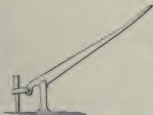
463a. STAKE PULLER. — An easy way to pull stakes and posts. A clevis to pinch the stake or post against the end of the lever with the lever pivoted to the foot post.
