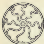
851. SPRING WHEEL.—Two forms of curved spring spokes and spring rim.
