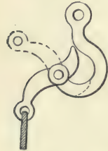
810. BOAT DETACHING HOOK.—The standard is fastened to the boat. A tongue is pivoted to its upper end and passes through the hook of the tackle-block. A lever with an eye to catch the tongue is pivoted to the upright standard, with a lanyard attached at the bottom. A simultaneous pulling of the two lanyards detaches both ends of a boat at once.
