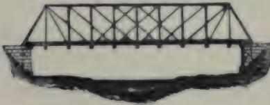
1490. BRIDGE TRUSS.—Vertical struts except in end panels, which have vertical tie rods. Inclined end struts and diagonal tie rods.
