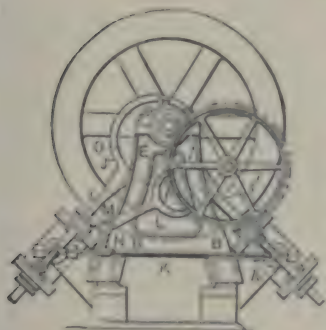
229. OSCILLATING HOISTING ENGINE.—The piston rods are attached to an eccentric strap; one fixed, the other pivoted. A lever operated by the same eccentric strap, through a short connecting rod, operates the valve gear of each cylinder alternately.
