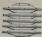
1145. COMPOUND DISC SPRING.—The discs are dished and perforated for a guide pin.
