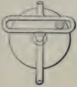
1039. SLOTTED YOKE CRANK MOTION, producing rectilinear motion of piston rod from a crank dispensing with a connecting rod.
