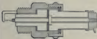
463f. ELECTRIC IGNITION PLUG, for a gas or gasoline motor. Electrodes of platinum; copper spindle with collar; insulation porcelain or lava with mica disk between.
