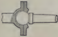
1396. BALL SOCKET, used on surveyor's compasses. The gland is tightened with countersunk screws.
