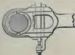
461. CONNECTING ROD END with locknut key.
