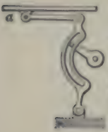
1042. INTERMITTENT RECIPROCATING MOTION from continuous circular motion. The curved slot in the lever should be radial with the crank centre for a stop. Many forms of motion may be had by variation of this device. A combination much in use for sewing-machines and printing-presses.
