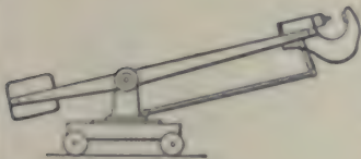
1456. BALANCED RIVETING MACHINE on a truck. For yard service, and iron and steel structural work.
