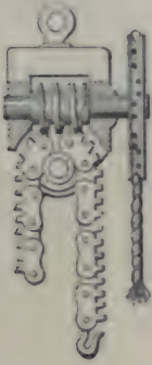
992a. LINK CHAIN HOIST.—A novel form of light weight hoists over lathes and planers. A screw gear working in a tooth chain.
