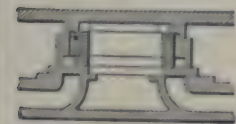
239. BALANCED SLIDE VALVE.— A ring in a recess of the valve rides against the steam chest cover, held by a spring.
