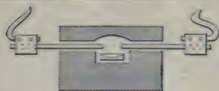
746. ELECTRIC FURNACE, showing the recess and flat crucible. Electrodes of hard carbon and connections.
