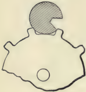
1059. INTERMITTENT MOTION of a toothed wheel by the revolution of a pinion with a single recessed tooth.
