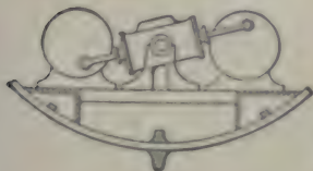
228. TWIN-SCREW OSCILLATING ENGINE.—A through piston rod connects directly to crank-pins on the shaft face plates. Suitable for small boats.
