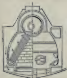
190. "YARROW" WATER TUBE BOILER.—Inclined sections of straight tubes from water-headers each side of the fire grate to a large steam drum above. Iron casing lined with fire tile. This design is for a marine boiler.
