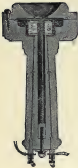
736. TELEPHONE RECEIVER.—A central magnet, with a coil of fine insulated wire around the end, next the vibrating plate or diaphragm. The variations in the electrical current produce variations in the intensity of the magnet, which set up vibrations of sound in the iron diaphragm.
