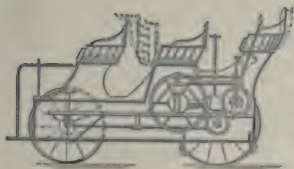
857. GASOLINE MOTOR CARRIAGE.—Two full seats and single seat for driver. The middle seat turns over to get at the motor and gear.
