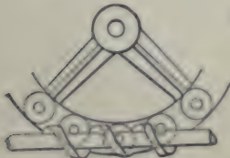
918. RELEASE ROTARY MOTION.—A worm wheel B, fast on a shaft to which is attached a loose arm and weight D, that carries the arm quickly over a half-turn, more or less, as required. The worm wheel lifts the arm and weight to beyond the vertical position by a pin in the shaft. See 919.
