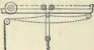
1406. TRAVELLER HOIST, showing the principles of the balanced counter pull and the traverse tackle.
