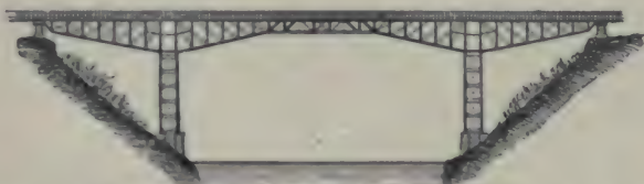
1505. CANTILEVER BRIDGE.—The ends, being anchored, balance all other parts on the piers. This cut shows the principle of Cantilever construction.
