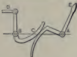
1077. WIPER CAM for stamp mills. A, the wiper; D, flanged chock, allowing the hammer spindle to revolve. Also in use on sewing-machines for throwing the needle bar
