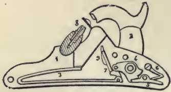
1638. GUN LOCK.—1, lock plate; 2, hammer; 3, mainspring; 4, tumbler; 5, sear or trigger lever; 6, sear spring.
