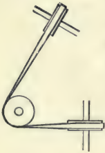
86. BELTING TO A SHAFT AT ANY ANGLE.— The two idler pulleys must be placed on a shaft at right angles to the driving and driven shafts, with their peripheries at the central line from centres from the driving and driven pulleys.
