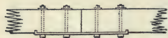
1481. TIMBER SPLICING.— Compression beams butted and held by a fish plate and bolts.
