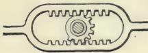
889. SECTOR PINION AND DOUBLE RACK.— Rectilinear reciprocating motion from the continual motion of a sector pinion.
