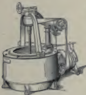
1145a. HYDRO - EXTRACTOR, showing method of belting with adjustable idler and cone pulleys.
