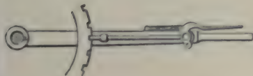
267. STARTING LEVER, with spring to hold the bolt in the sector notches.
