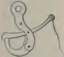
1455. TRIP HOOK.—A split shank with tongue and catch pivoted between the sides of the shank as shown.
