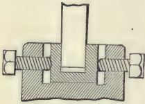
1279. VERTICAL SHAFT STEP.—Made adjustable by a movable bearing held by set screws in the foot block.
