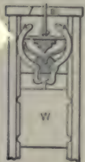
1457. RELEASING GRIP of a pile-driving machine. The bow ends of the grip are compressed when they reach the slot B in the frame and cast off the ram W. The springs between the bowed handles of the grip close the jaws to pick up the ram.
