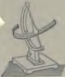
1543. MEAN TIME SUNDIAL.—The length of the stile is made to just cover the entire range of the sun's altitude at the distance of the scale on the hour circle. Its shape and size to be proportionate to the sun's equation of time as marked on the scale. When the sun is fast the reading should be on the left-hand side of the shadow, and when slow on the right side.
