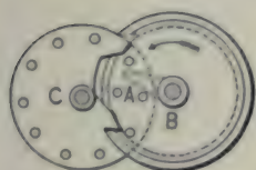
166. INTERMITTENT ROTARY MOTION, for counters and meters. B, driving wheel, the rim of which has an entering and exit notch for pins in the driven wheel and locks the wheel C at each revolution of wheel B.
