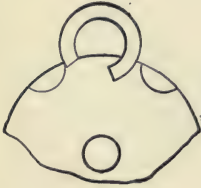
1057. INTERMITTENT MOTION of a segmental-toothed wheel by the revolution of a segmental barrel or ring.
