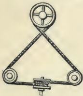
59. TRANSMISSION BY ROPE to a shaft at right angles to the driving-shaft. The guide sheaves give direction to the rope over the curve face of the driven pulley, the rope slipping towards the centre of the driven pulley.
