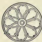
852. ELASTIC WHEEL, with steel tire and spring spokes.
