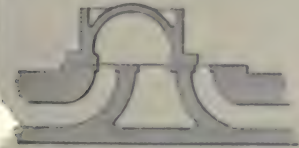
238. SINGLE D SLIDE VALVE, with lap. The length of the valve over the length from outside to outside of steam ports is double the lap.
