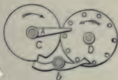
165. INTERMITTENT ROTARY MOTION, for counters and meters. The tappet A, revolving with the wheel C, carries the wheel D one pin notch per revolution. The pawl b is released by the notch in the wheel C while the tappet is in contact with the pin.
