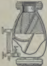
404. STEAM SEPARATOR. — The entrained water in the steam is lodged upon the rough walls, and drips to the strainer and into the pocket, and is drawn off through the valve. The glass gauge indicates the height of water in the pocket.
