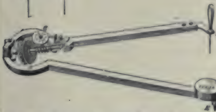
155. "AMSLER" PLANIMETER.—E is the fixed point; F the tracer. The disc has a sharp edge and a cylindrical section divided and read from a vernier scale. A worm screw and index wheel indicate the number of revolutions of the rolling disc.
