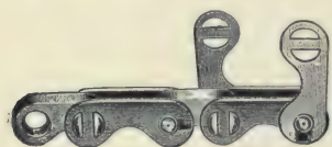
871. DETACHABLE LINK CHAIN for bicycles. Chain can be taken apart by turning the links at right angles to the run of the chain.
