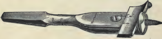
1391. EXPANSION BIT.—The spring clip held by a screw clamps the cutter in position
