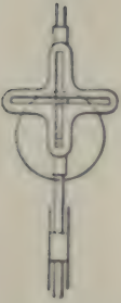
1040. TRAMMEL GEAR.—The slotted cross moves in a right line astride the shaft, while the crank pin in a block moves in the cross slot.
