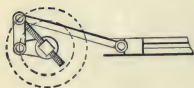
1126. VARIABLE CRANK THROW. —The jointed crank and radial screw give a large variation to the throw of a crank.
