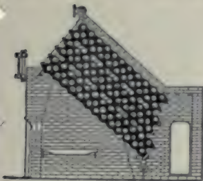
185. "HARRISON" BOILER.—A series of cast-iron globes with ground joints, held together by through bolts.
