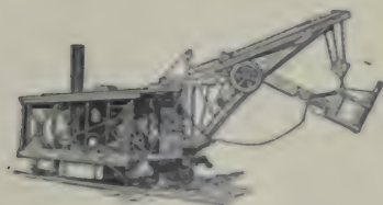
1254. RAILWAY STEAM SHOVEL, the "Victor" model. For excavating railway cuts, or general work on temporary rails.
