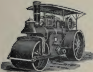
848. ROAD ROLLER.—Steam-driven. One of the heavy class now improving our roads.
