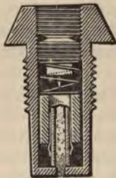
FIG. 50.—At the start of a shell the fuse is primed, and on its arrival the striker fires the charge.
