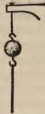
FIG. 48.—A slow pull breaks the upper wire, a jerk the lower. In the first case, the ball acts by its weight; in the second, by its mass.
