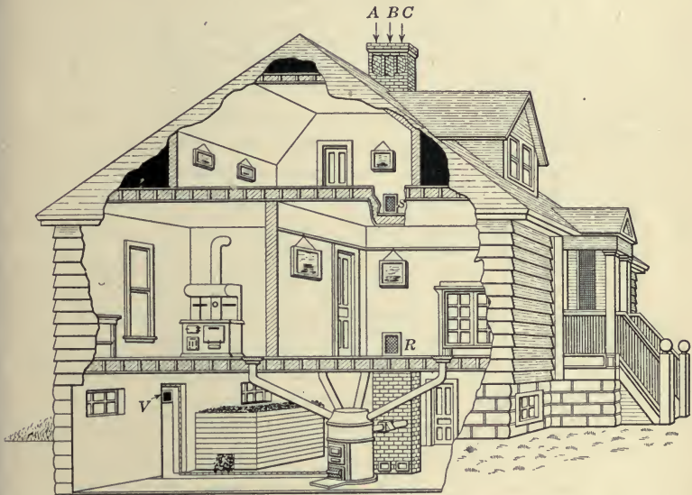
FIG. 163.—A chimney flue used as a ventilator.
