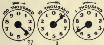
FIG. 177A.—Gas-meter dial. It reads 38600 cubic feet.
