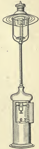
FIG. 200.— Boulevard lamp with generator in the base of the lamp post.
