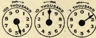
FIG. 177B.—Gas-meter dial. It reads 40100 cubic feet.
