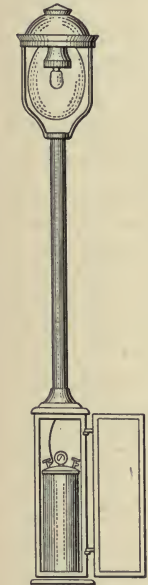
FIG. 201.— Boulevard lamp operated by the hollow-wire method of light- ing.
