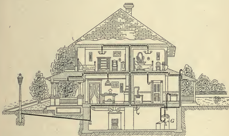
FIG. 212.—Sectional view of a house equipped with acetylene lights and domestic heating apparatus.
