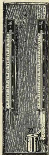
FIG. 157.—Hygrometer of U. S. Weather Bureau type; for determining atmospheric humidity.
