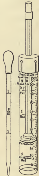
FIG. 165.—The Wolpert air tester; an instrument used to determine the quality of air.
