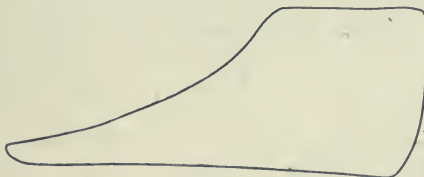
Fig. 7. Crank end. Card shown, one-half size; area of original, 4.62 square inches; stiffness of spring, 50 pounds per square inch; length of stroke 30 inches; revolutions per minute, 84; piston diameter, 13\frac{1}{2} inches.
