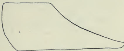
Fig. 6. Head end. Card shown, one-half size; area of original, 4.69 square inches; stiffness of spring, 50 pounds per square inch; length of stroke, 30 inches; revolutions per minute, 84; piston diameter, 13\frac{1}{2} inches.
