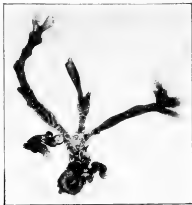
FIG. 40.—Osmotic growth in a solution of \text{KNO}_3 , showing spine-like organs.
