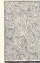
Asbestos or Fiber.
