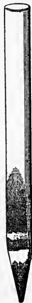
Fig. 48.—Ordinary reduction-tube, with two sublimate; the upper, brownish black; the lower, the pure metal in an annular deposit.
