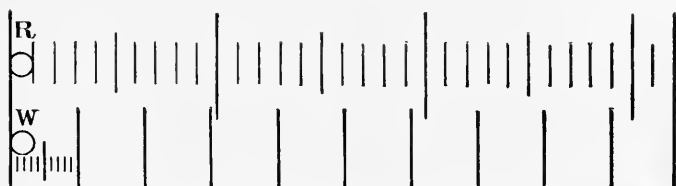
Fig. 16.—Lines of eyepiece micrometer, projected upon stage micrometer, as seen with different magnification.
