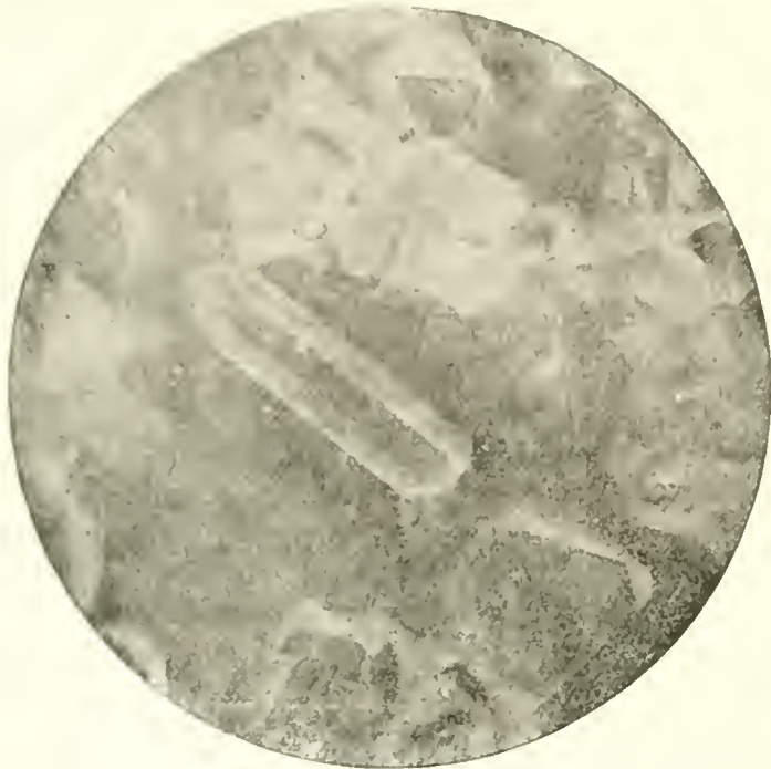
FIG. 9.—Prismatic Crystal of Arsenic Trioxid, among Octahedra. By Sublimation in Sulfur Dioxid. \times 250 .
