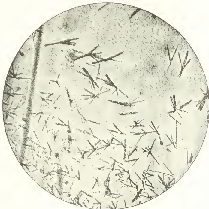
FIG. 18.—Reinsch Test. Antimony, Amorphous and Prismatic Deposit with a few Octahedra. \times 75 .
