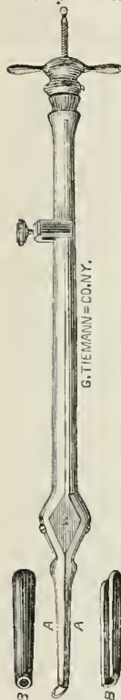
A, A, Fingers. B, B, Gloves of hard rubber. W, Wedge which separates the fingers.
