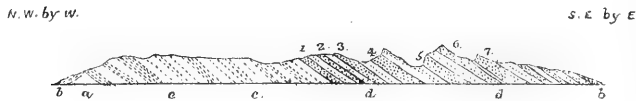
Fig. 6.—Section across the Alicoor hills, from north-west by west to south-east by east. a, Gneiss; c, Sripermatoor group; d, Sattavedu group; e, talus. Nos. 1—7. Conglomerate beds.
