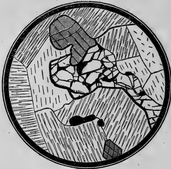
Fig. 4—Crystal of olivine, partially enveloping green augite in laurvikite. Rock No. 11,463, magnified by 40 diameters.
