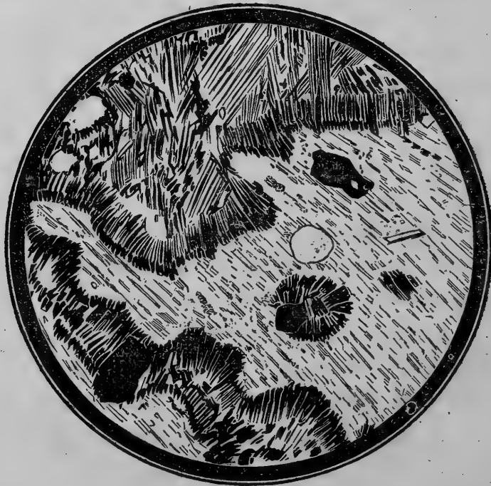
Fig. 1.—Altered biotite-gneiss near its contact with charnockite, 3\frac{1}{2} miles south of Salem. (Section magnified by 20 diameters.)
