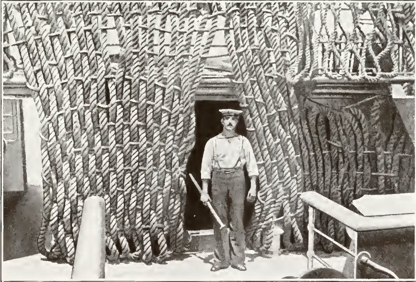
ROPE PROTECTION ON "CARMANIA" AGAINST SHELL SPLINTERS
