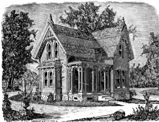
Front Elevation of a Gothic Suburban Residence. First story 13 feet; second story 10 feet, in clear.
