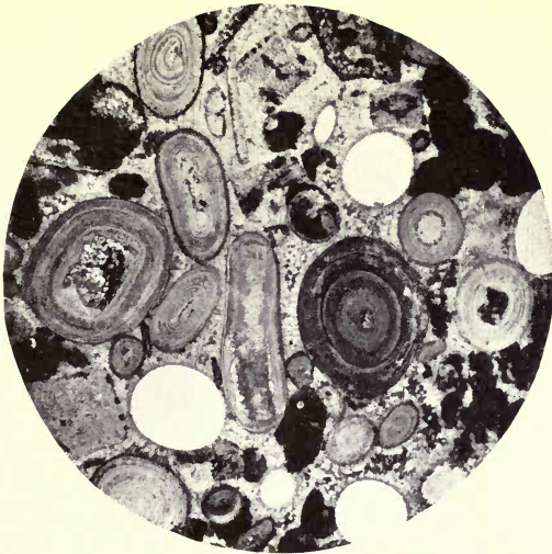
1. TYPICAL EXAMPLE OF RAASAY GREEN ORE FROM MAIN MINE, RAASAY. (Ordinary light, magnified 11 diameters.)
