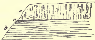
Occurrence of copper ores in the New Red Sandstone. a , Trap; b , Sandstone; c , Copper ores.
