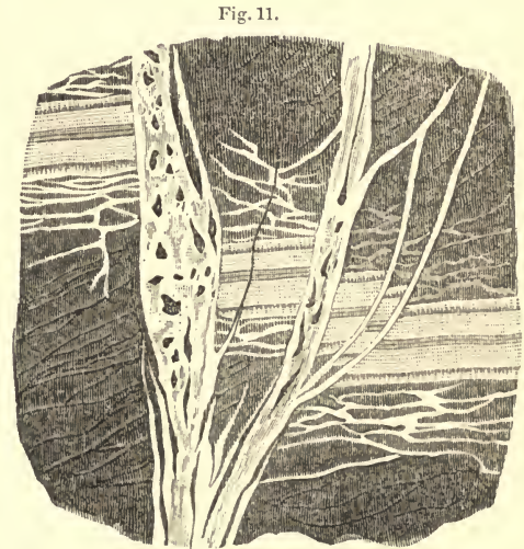
Ground plan of the intersection of veins in the Himmelfahrt mine, near Freiberg.
