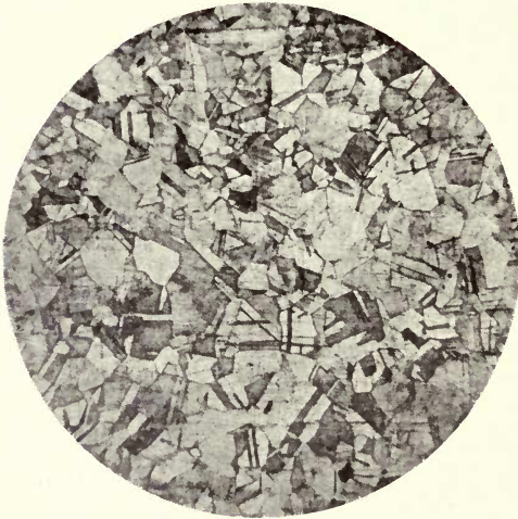
B. Brass (Cu 70, Zn 30%) annealed. \times 86 .
