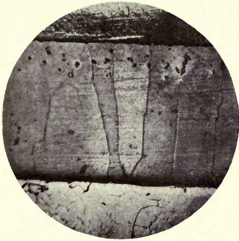
A. Diffusion of zinc into copper. \times 30 .
