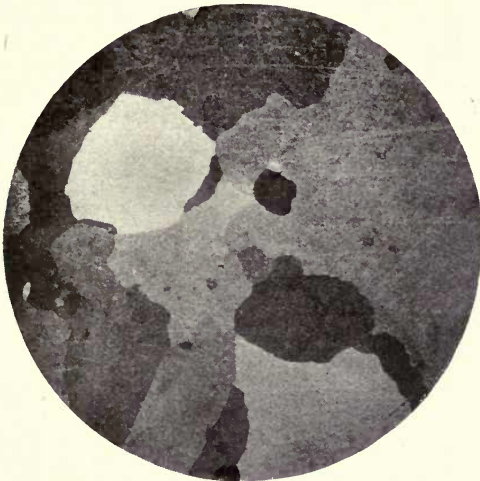
B. Etched surface of cast tin. \times 4 .
