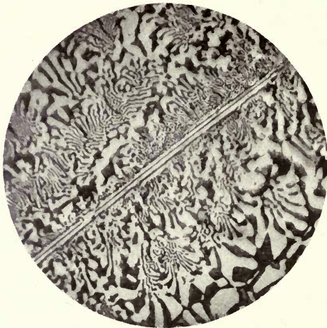
B. Eutectic of copper and copper phosphide. \times 200 .
