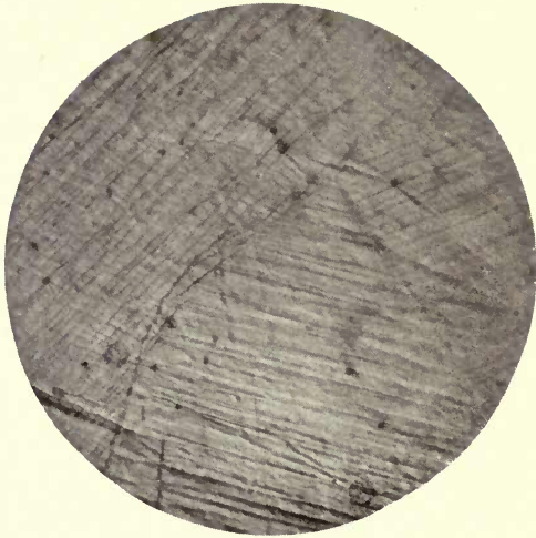
A. Strained surface of lead, showing slip-bands. \times 86 .
