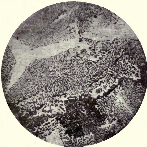
B. Alloy of bismuth, lead, and tin. \times 200 .
