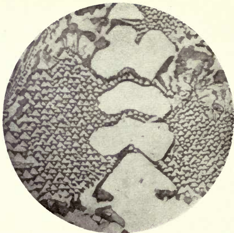
A. Alloy of antimony and \text{Cu}_2\text{Sb} . \times 200 .
