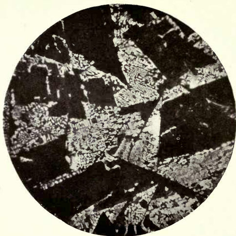
A. Copper 55, aluminium 45%. \times 86 .
