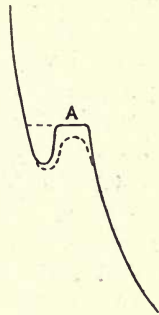
FIG. 74.—Effect of undercooling on cooling curve.
