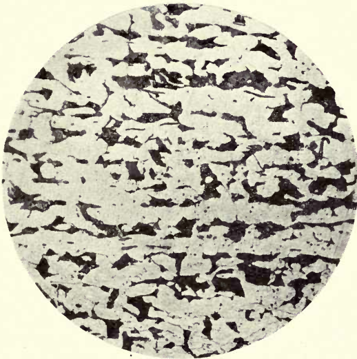
B. Mild steel plate. \times 250
