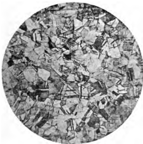
B. Brass (Cu 70, Zn 30%) annealed. \times 86 .
