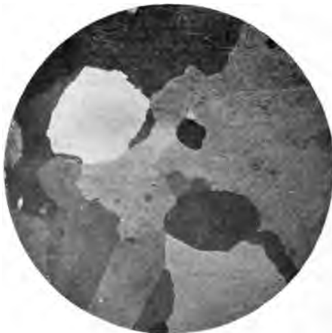
B. Etched surface of cast tin. \times 4 .
