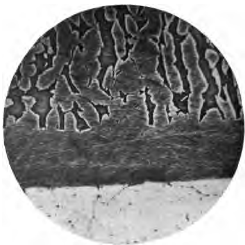
B. Diffusion of zinc into copper. \times 30 .
