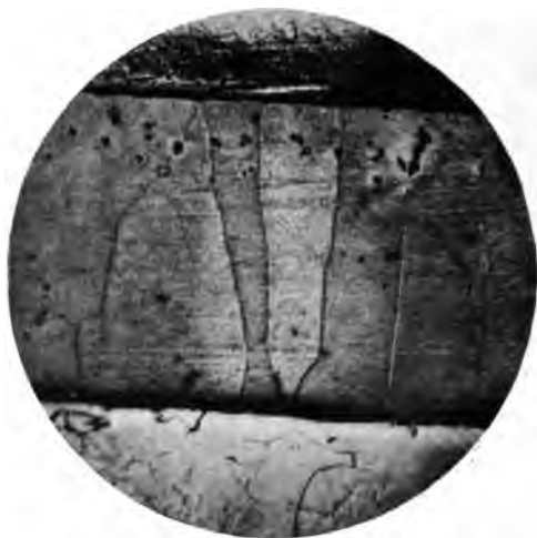
A. Diffusion of zinc into copper. \times 30 .
