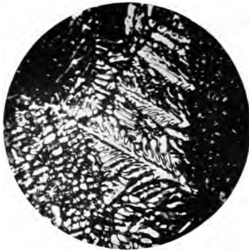
A. Surface of cast tin. \times 15 .
