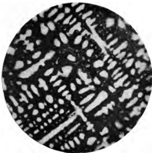
A. Copper 50, nickel 50%. \times 86 .
