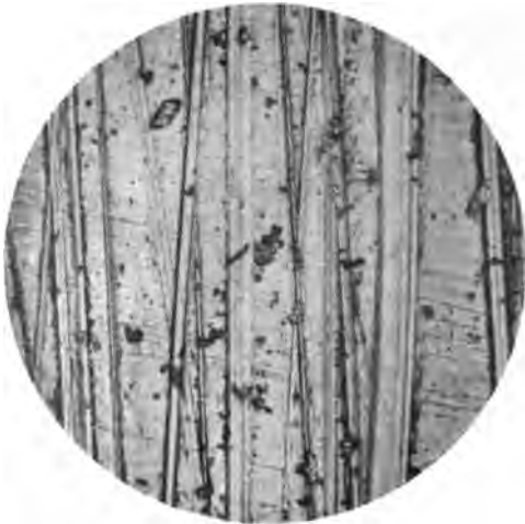
A. Surface of bismuth, marked with emery scratches. \times 200 .
