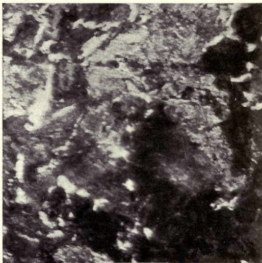
FIG. 47.—The same cemented steel as in Fig. 46. Magnified 650 diameters. Photograph taken near the edge of the carburetted zone.
