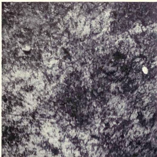
FIG. 68.—High-speed Steel. C = 0.58 per cent. W = 10.2 per cent. Cr = 8.3 per cent. Magnified 300 diameters. Acted upon by aqua regia.
