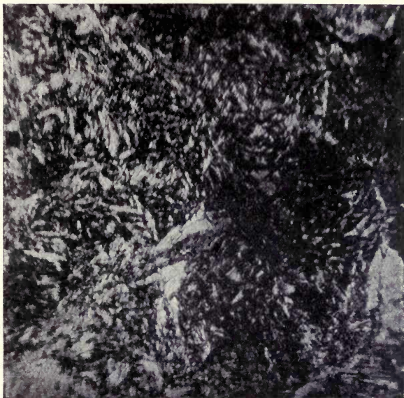
FIG. 42.—75 per cent. steel, tempered at 800^{\circ} in water. Magnified 650 diameters. Acted upon by Kourbatoff's reagent.
