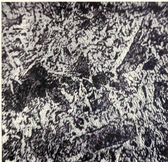
FIG. 51.—C = 0.25 per cent. Ni = 7 per cent. Magnified 650 diameters. Acted upon by 5 per cent. picric acid.
