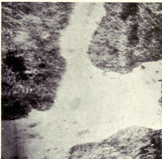
FIG. 27.—Crude Steel with 0.455 per cent. carbon. Magnified 550 diameters. Acted upon by Kourbatoff's reagent.
