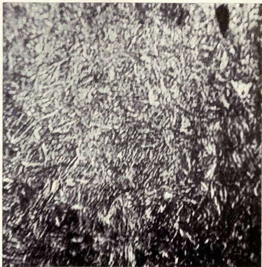
FIG. 54.—C = 0.25 per cent. Ni = 15 per cent. Magnified 650 diameters. Acted upon by 5 per cent. picric acid.
