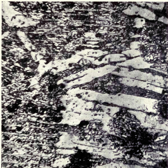
FIG. 12.—Cementite (the light part), in a steel soldered under the oxyacetylenic blowpipe. Magnified 650 diameters. Acted upon by 4 per cent. nitric acid in amylic acid.
