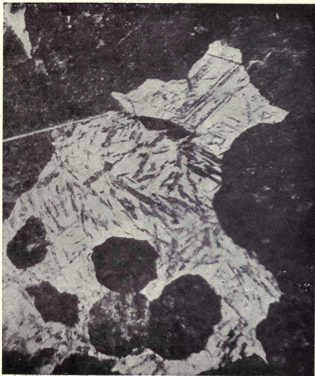
FIG. 92.—Partially tempered Steel. Martensite, troostite and sorbite. Magnified 650 diameters. Acted upon by Kourbatoff's reagent.
