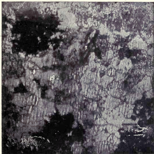
FIG. 88.—Malleable Cast-iron of group III. (see Table), annealed in sand and oligoschist. Magnified 300 diameters. Acted upon by Kourbatoff's reagent.
