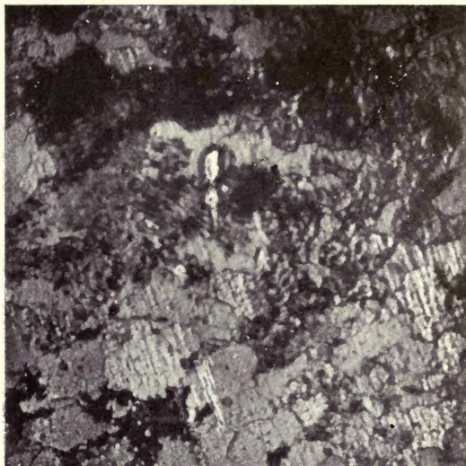
FIG. 89.—Malleable Cast-iron of group III., annealed in pure sand. Magnified 300 diameters. Acted upon by Kourbatoff's reagent.
