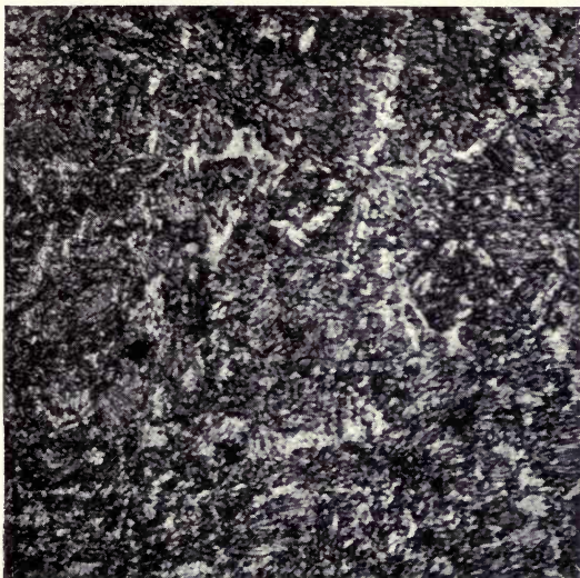
FIG. 65.—The same steel as in Fig. 64, tempered at 800° C. in water. Magnified 300 diameters. Acted upon by 5 per cent. picric acid.
