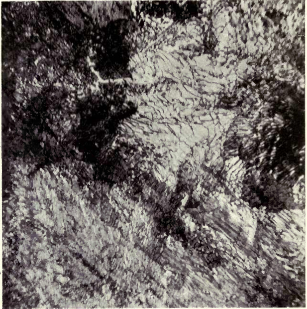
FIG. 31.—Crude Steel, C = 0·75 per cent. Magnified 650 diameters. Acted upon by Kourbatoff's reagent.
