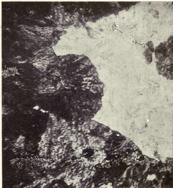
FIG. 93.—Partially tempered Steel. Martensite and sorbite. Magnified 650 diameters. Acted upon by Kourbatoff's reagent.
