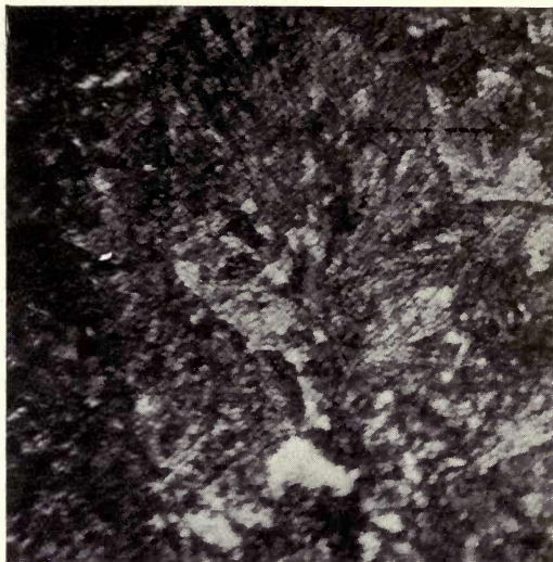
FIG. 45.—Extra hard steel softened at 300^{\circ} , sorbite and remains of martensite in the centre. Magnified 300 diameters. Acted upon by 5 per cent. picric acid in ethylic alcohol.
