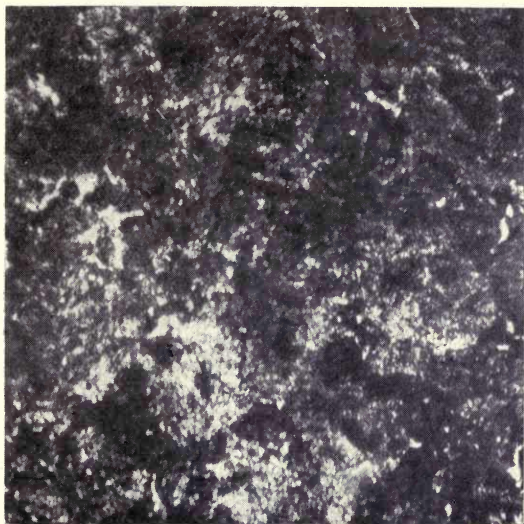
FIG. 48.—Cemented Steel with 0.6 per cent. carbon. Magnified 150 diameters. Photograph taken in the middle of the sample.
