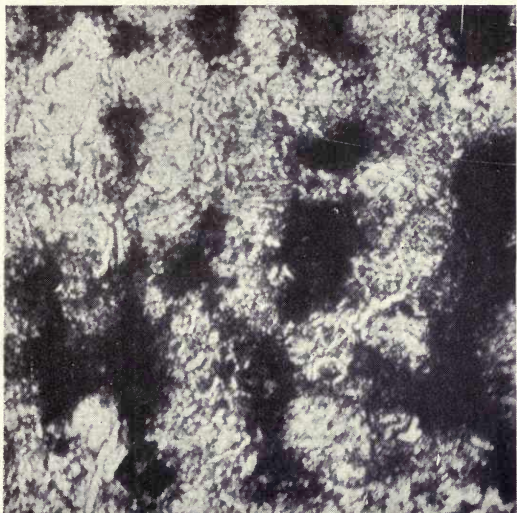
FIG. 76.—Malleable Cast-iron, obtained by annealing the white cast-iron of Fig. 69. Outer portion, ferrite and graphite. Magnified 300 diameters. Acted upon by 5 per cent. picric acid.
