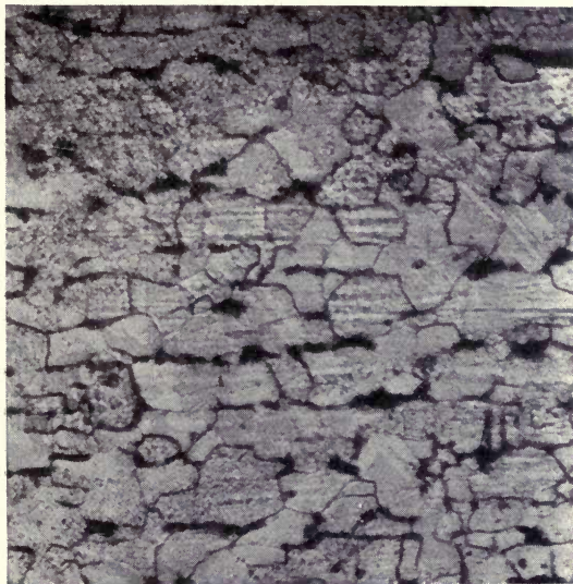
FIG. 21.—Rolled Iron, cut in the direction of the rolling. Magnified 300 diameters. Acted upon by Kourbatoff's reagent.
