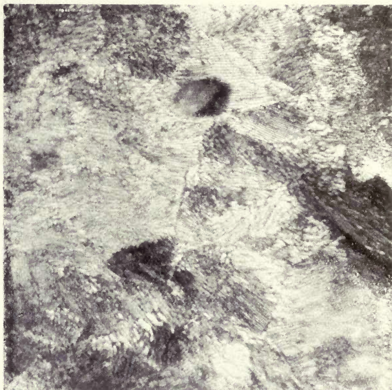
FIG. 16.—Pearlite and Sorbite (dark spots) in steel at 0.85 per cent. Magnified 650 diameters. Acted upon by 5 per cent. picric acid.
