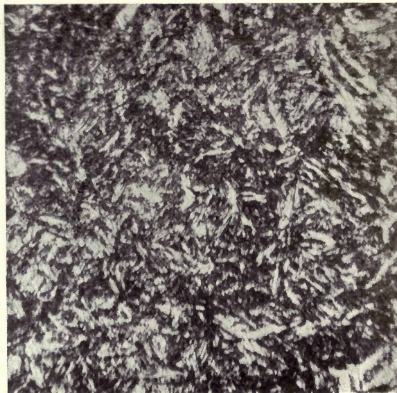
FIG. 43.—Steel with 0.85 per cent. carbon, tempered at 800° in water. Magnified 650 diameters. Acted upon by Kourbatoff's reagent.
