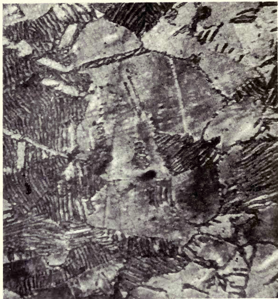
FIG. 63.—C = 0·8 per cent. Ni = 25 per cent. Magnified 650 diameters. Acted upon by 5 per cent. picric acid.
