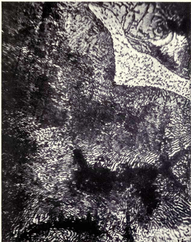
FIG. 72.—Phosphorous Grey Cast-steel. Magnified 150 diameters. Acted upon by Kourbatoff's reagent.
