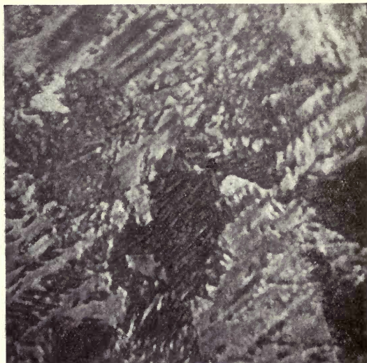
FIG. 56.—C = 0.25 per cent. Ni = 25 per cent. Magnified 650 diameters. Acted upon by 5 per cent. picric acid.
