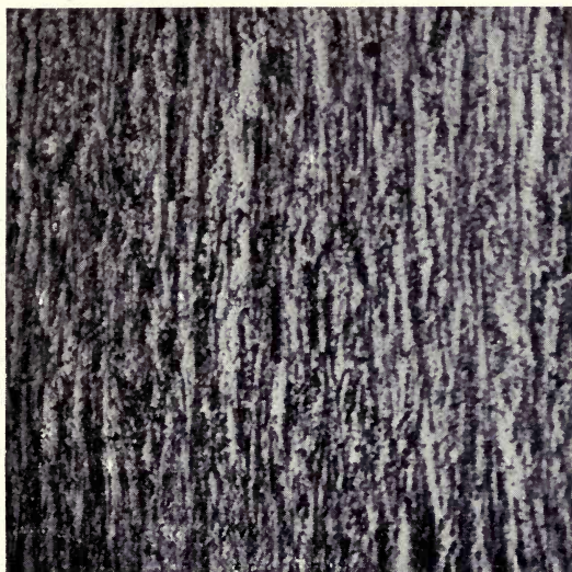
FIG. 36.—Hammer-hardened steel, C = 0.46 per cent. Magnified 300 diameters. Acted upon by Kourbatoff's reagent.
