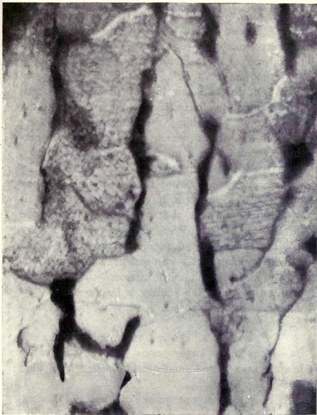
FIG. 20.—Iron puddled and rolled in the direction of the arrow. Magnified 1100 diameters. Acted upon by Kourbatoff's reagent.
