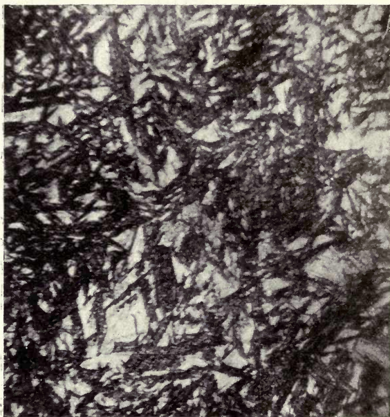
FIG. 61.—C = 0.8 per cent. Ni = 12 per cent. Magnified 650 diameters. Acted upon by 5 per cent. picric acid.
