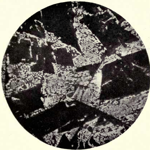
A. Copper 55, aluminium 45%. \times 86 .
