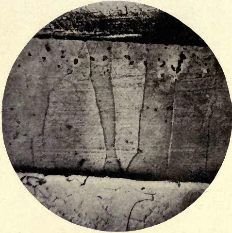
A. Diffusion of zinc into copper. \times 30 .
