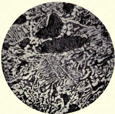
B. Eutectic alloy of bismuth and lead. \times 200 .
