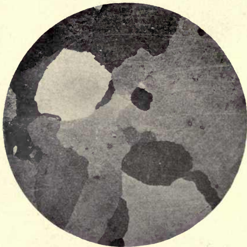
B. Etched surface of cast tin. \times 4 .
