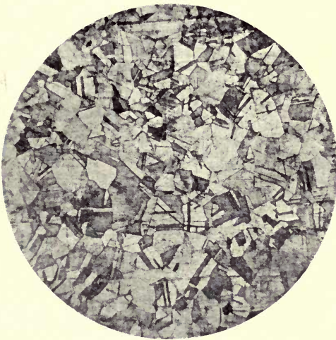
B. Brass (Cu 70, Zn 30%) annealed. \times 86 .
