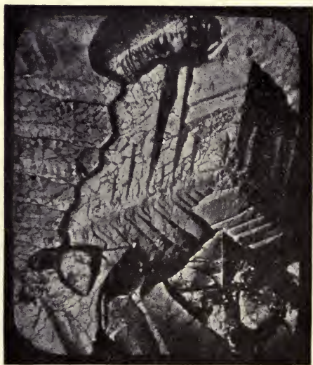
FIG. 164.—Internal Dendritic Structure ( \times 40 ).
