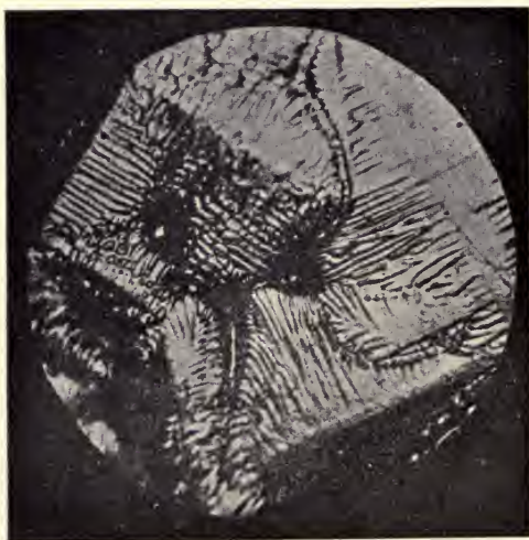
FIG. 46.—Surface of Fused Platinum ( \times 33 ).
