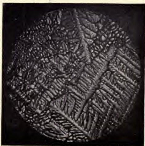
FIG. 158.—Surface of Impure Tin ( \times 33 ).
