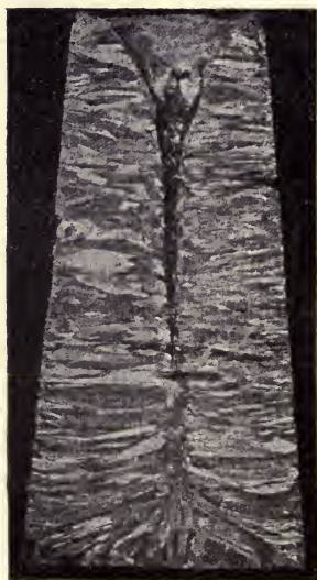
FIG. 215.—Structure of Bar Zinc.
