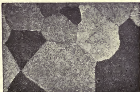
FIG. 160.—Large Grains caused by Tempering Tin.
