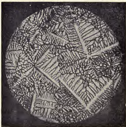
FIG. 217.—Dendritic Structure on Lower Side of Cast Ingot.
