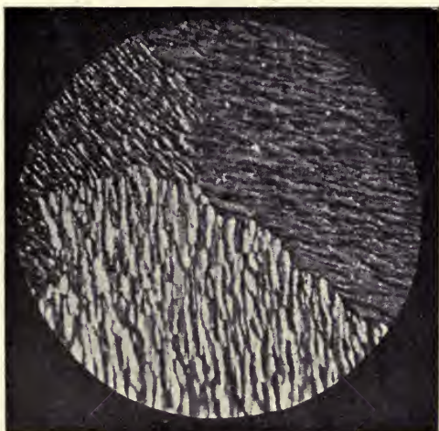
FIG. 159.—Deeply Etched Under-surface of a Cast Tin Ingot.
