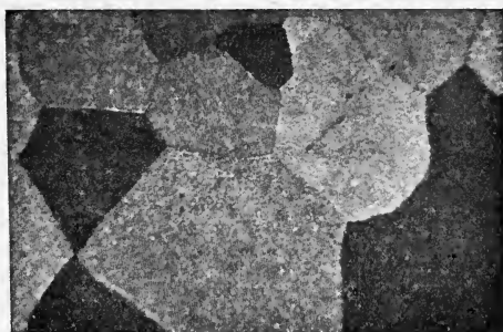
FIG. 160.—Large Grains caused by Tempering Tin.
