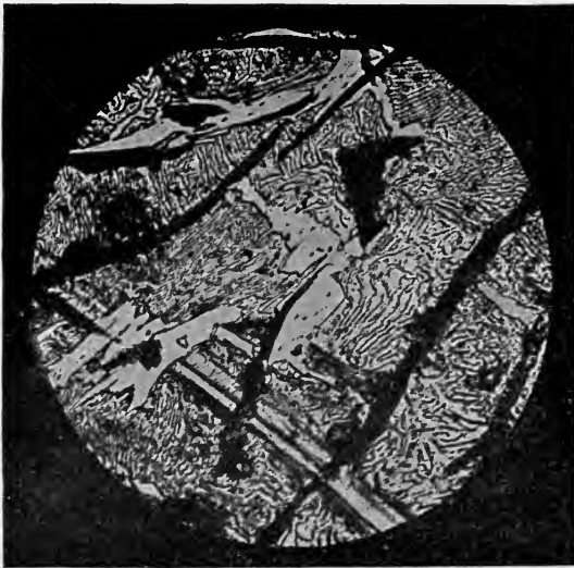
FIG. 179.—Gray Cast Iron. Graphite (Black); Cementite (White) with Lamellar Pearlite ( \times 500 ).
