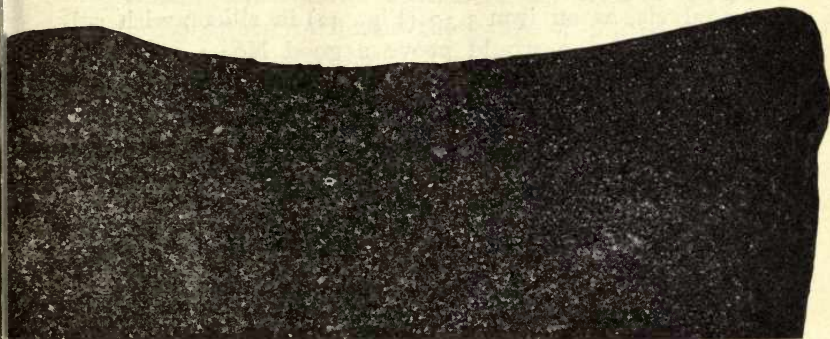
FIG. 41.—NO. 7 IRON BY FRACTURE, BUT NO. 4 BY ANALYSIS.
