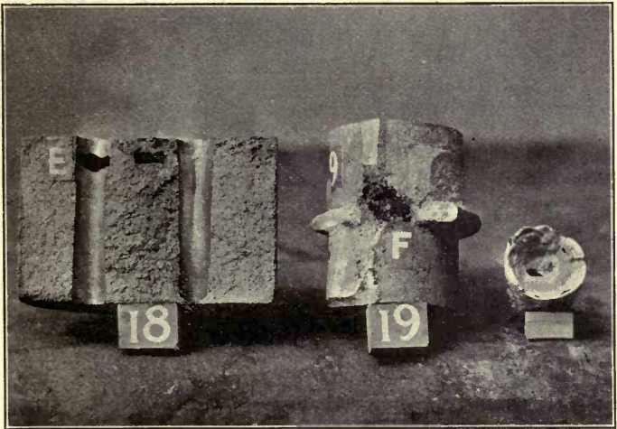
FIG. 80.—CASTINGS SHOWING TYPICAL POSITIONS OF SHRINK HOLES.
