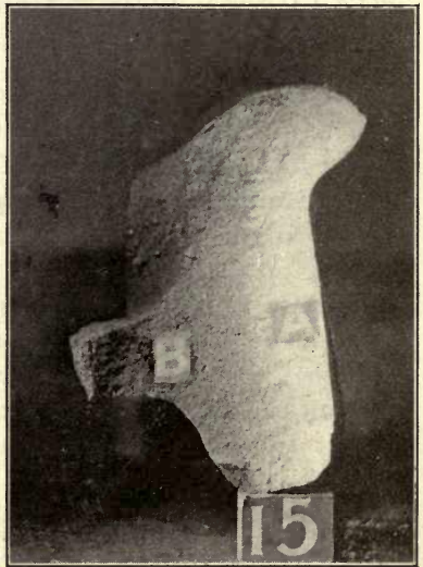
FIG. 57.—SECTION OF CHILLED CAST IRON CAR WHEEL.
