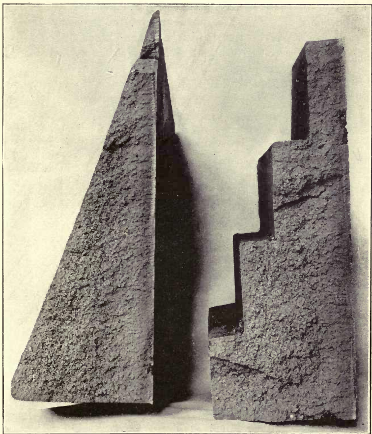
FIG. 146.—FRACTURE OF CHILL TEST PIECES IN SERIES B.
