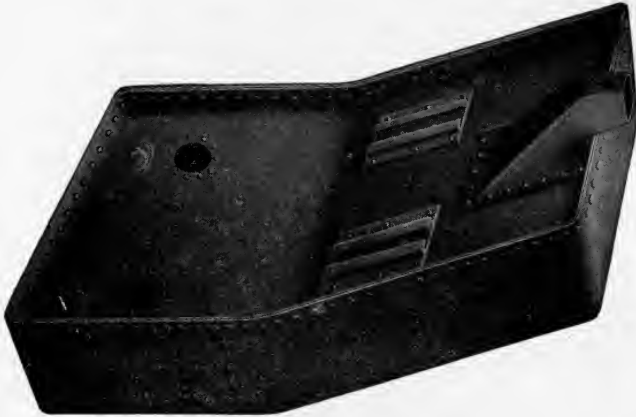
Fig. 159. END WATER-JACKET, WITH KNEE-BOSH.
