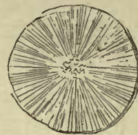
Fig. 27.—Columnar structure of ingots. Chernoff.
