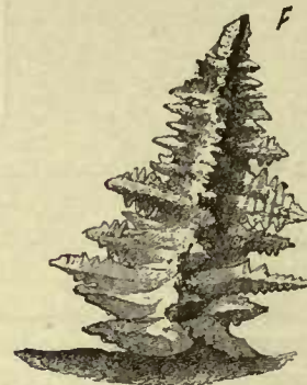
Fig. 31. Pine-tree crystal from iron. Knop.
