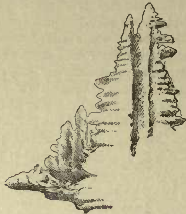
Fig. 29.—Crystal from a pipe in steel. Magnified 70 times. Chernoff.
