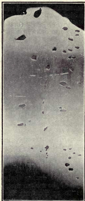
FIG. 27. BLOW-HOLES IN NICKEL STEEL INGOT.
