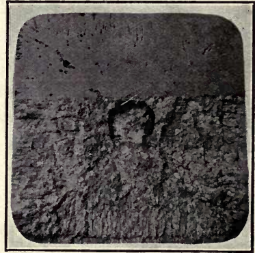
FIG. 22. "PIPE" IN NICKEL STEEL INGOT.
