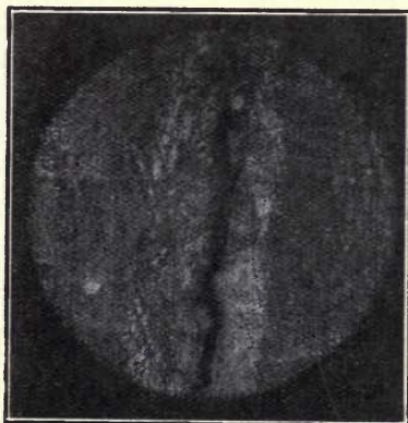
FIG. 25. MICROPHOTOGRAPH OF " PIPE " IN TENSILE TEST-PIECE.
