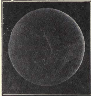
FIG. 33. CRUSHED CENTRE IN ROUND NICKEL CHROME STEEL BAR.
