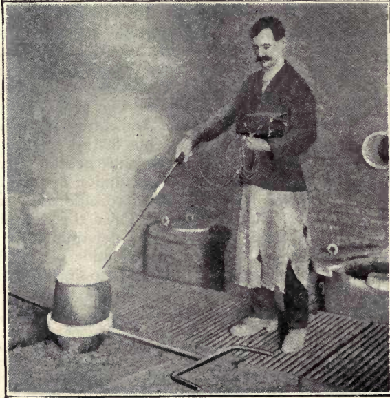
FIG. 47. TAKING THE TEMPERATURE OF MOLTEN METAL WITH THERMO-ELECTRIC PYROMETER.
