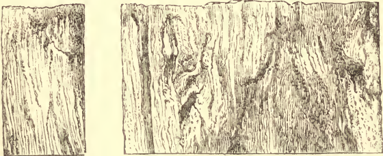
FIG. 19.--Structure of Puddled Bar.
