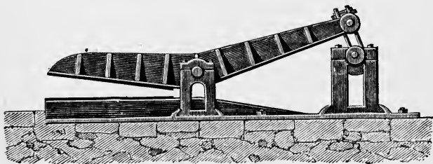
FIG. 13.—Squeezer for Puddled Balls.
