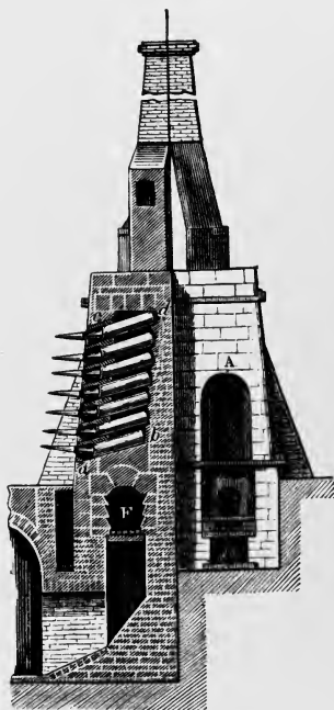
FIG. 56.—Belgian Furnace for distilling Zinc from its Ores.
