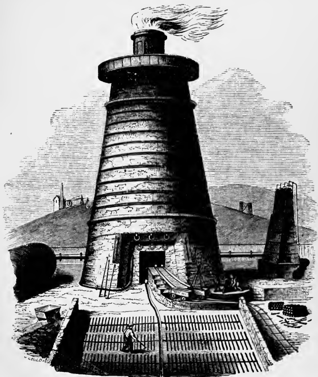
FIG. 5.—Hot-Blast Furnace for Smelting Iron Ores ; showing, on the right, the stove for heating the blast ; on the left, the large air-chamber or regulator for equalising the blast. In front are seen the slag-moulds on a tramway, and the channel through which the cast iron is conducted into the pig-moulds.
