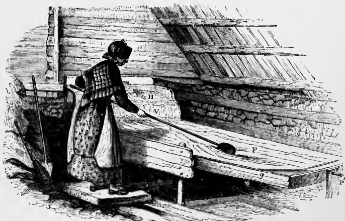
FIG. 46.—Rack for washing Ores.
