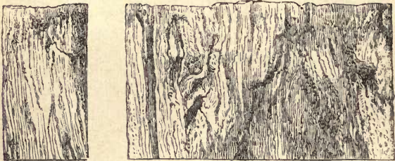
FIG. 19.--Structure of Puddled Bar.
