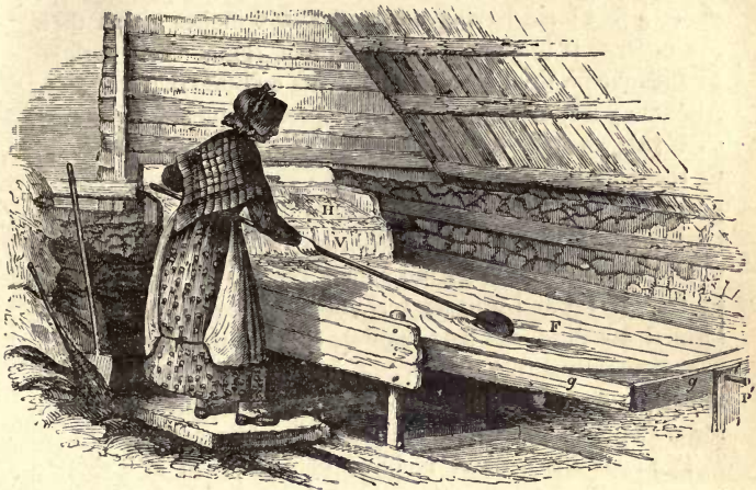
FIG. 46.—Rack for washing Ores.
