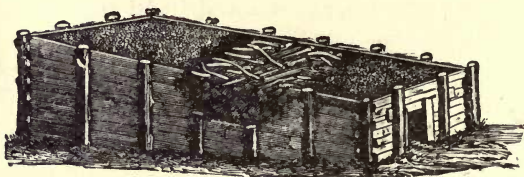
FIG. 2.—Rectangular Pile for Burning Charcoal.
