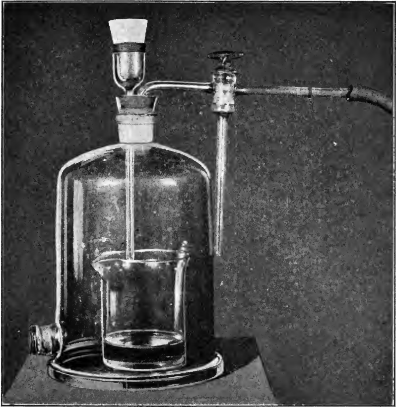
FIG. 4.—SUCTION FILTERING APPARATUS FOR REDUCING SUGAR DETERMINATIONS.
