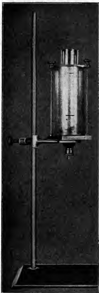
FIG 7.—FLOW VISCOSIMETER WITH WATER JACKET.
