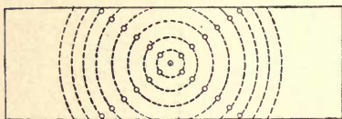
FIG. 48.—Cargo Sampling— The Cone.
