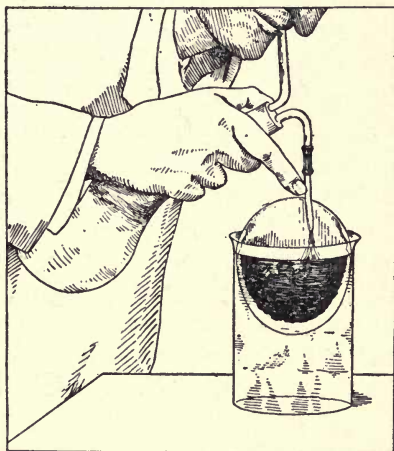
FIG. 52.—Washing a Precipitate from the Filter Paper to a Beaker.
