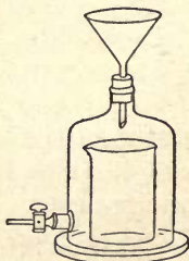
FIG. 27.—Bell Jar Arranged for Filtering by Suction Directly into a Beaker.
