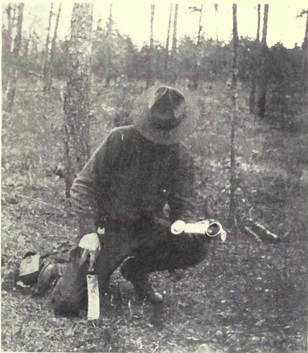
Fig. 66 Forest officer preparing to use the Adams hand set with Cree knife for ground rod
