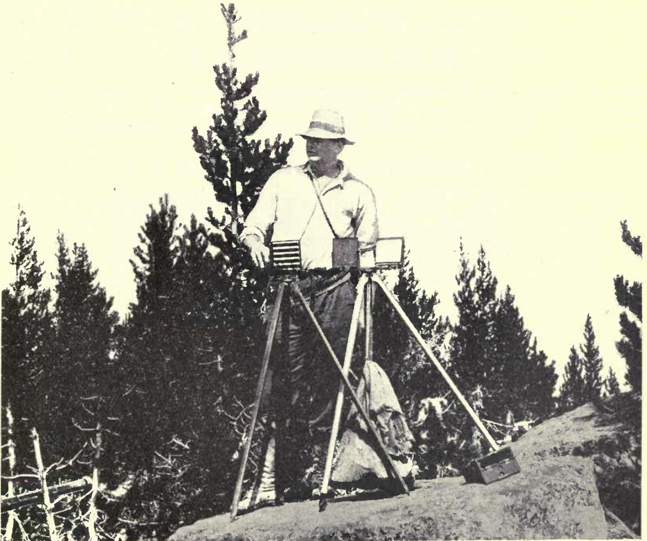
Fig. 105 Forest ranger sending message by heliograph
