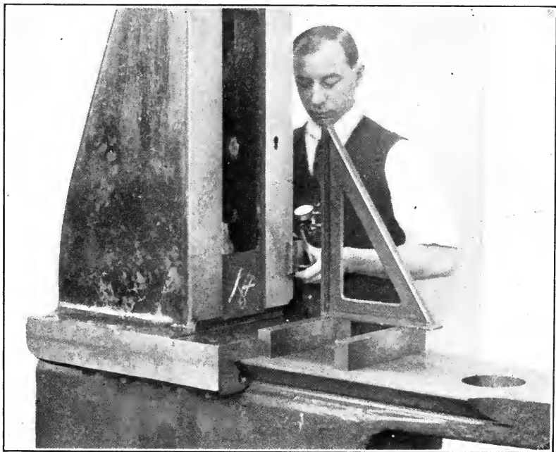
FIGS. 84 and 85.—Testing the squareness of a milling machine knee.
