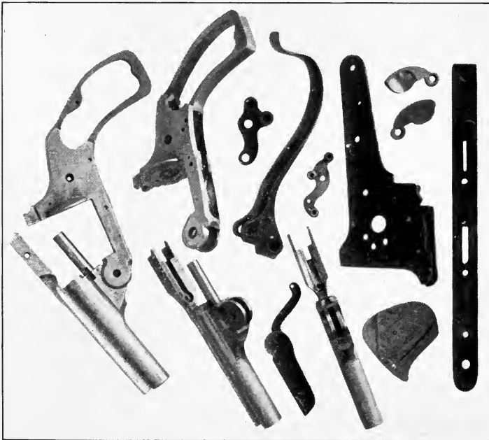
FIG. 243.—Work of the profiling machine.
